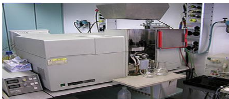
Fig. 8: Flame atomic absorption spectroscopy instrument (Wikipedia)
