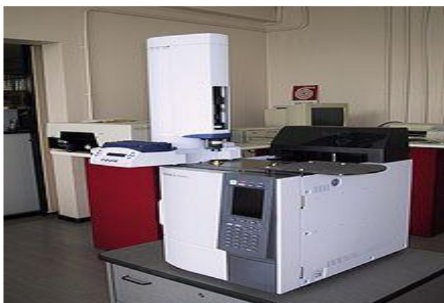
Fig. 18: A gas chromatograph with a headspace sampler
