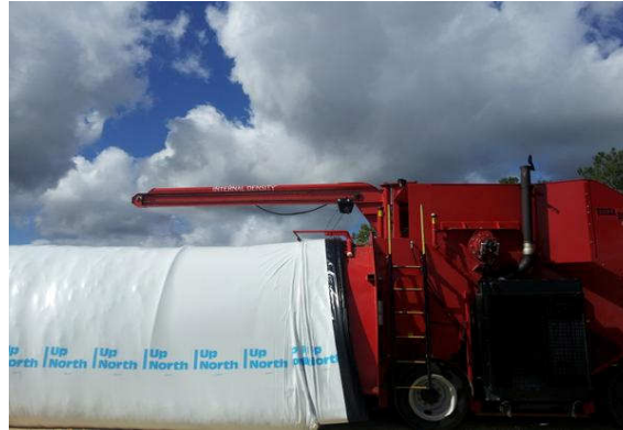
Figure 4. Bag silo filling.
