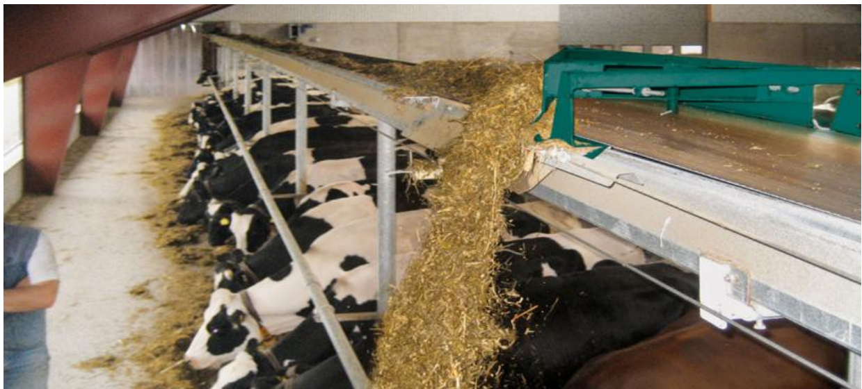
Automatic feed conveyor
