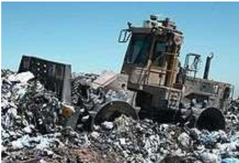
Fig. 5.3: A Landfill Compaction Vehicle in Action
