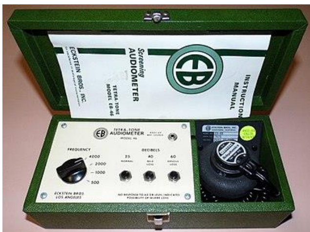
(a) Portable audiometer Tetra-Tone Model EB-46, circa 1975 (b) Portable audiometer Maico, circa 1960s-
