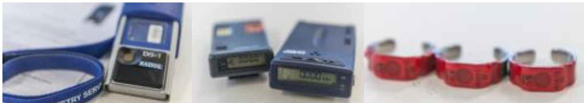
Figure (a) Personal dosimeter (b) Operational dosimeters (c) Extremity dosimeters
