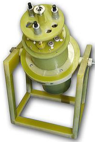
Figure 1: A non-metallic, tilt able bath cryostat for liquid nitrogen
