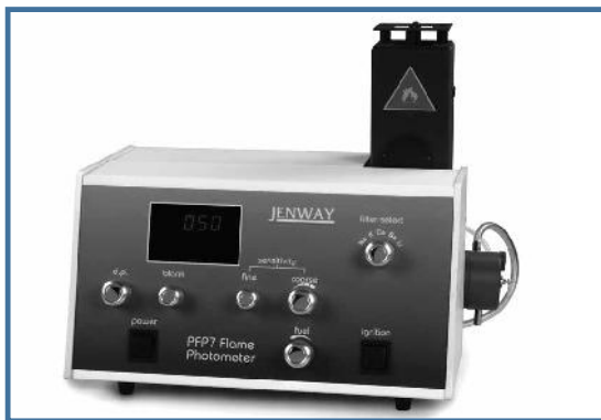
Fig. 3.4: Jenway Flame Photometer
