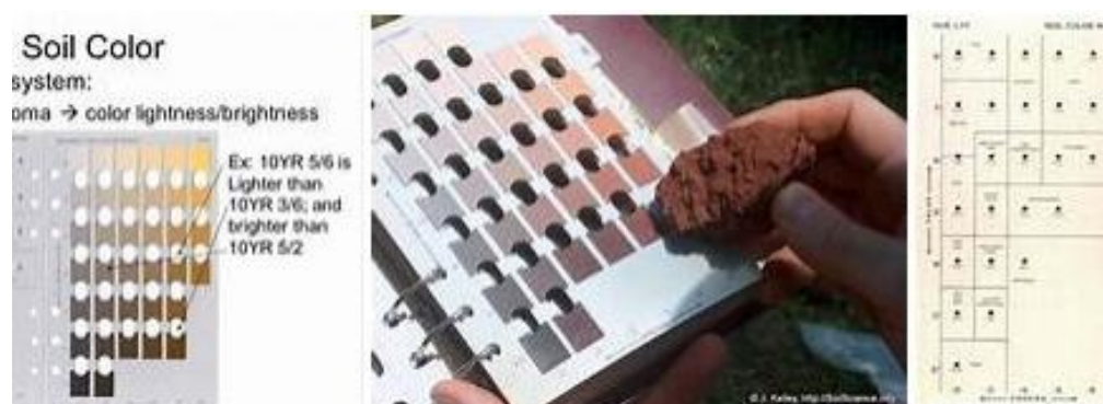
Fig. 6b: Soil Scientist using Munsell Colour Chart to detect soil colour
