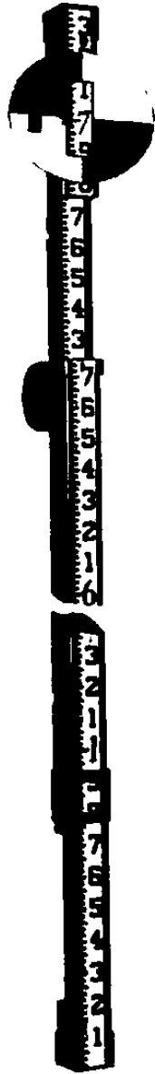
Courtesy of Keuffel and Esser A PHILADELPHIA-TYPE LEVELING ROD
