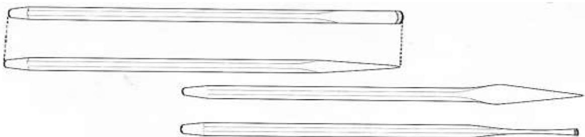
Fig. 77. Flat and cross-cut chisels for general work.
