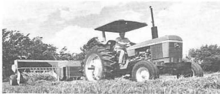
FIG. 16-2. Utility tractor, 70 h.p., pulling baler. (Courtesy Deere and Company)
