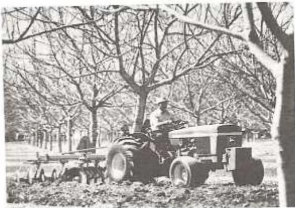
FIG. 16-9. Orchard tractor with low profile. (Courtesy Deere and Company)
