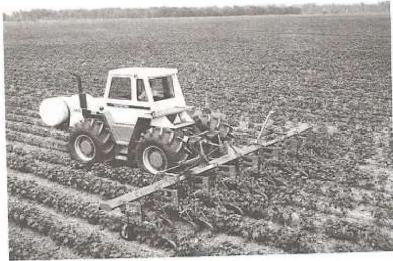
FIG. 16-8. Four-wheel drive tractor cultivating row crops. (Courtesy J. I. Case)
