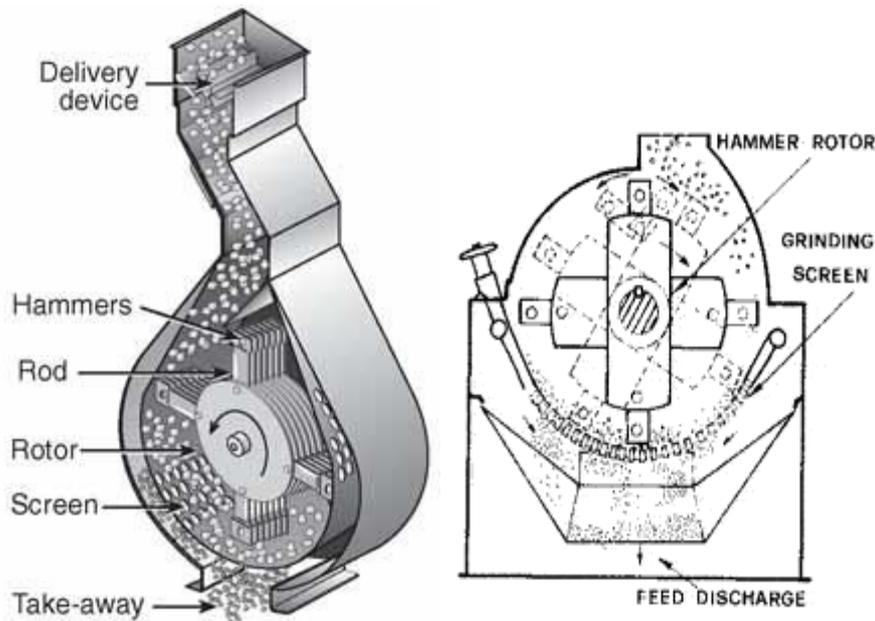
Diagram of a Hammer Mill Machine
