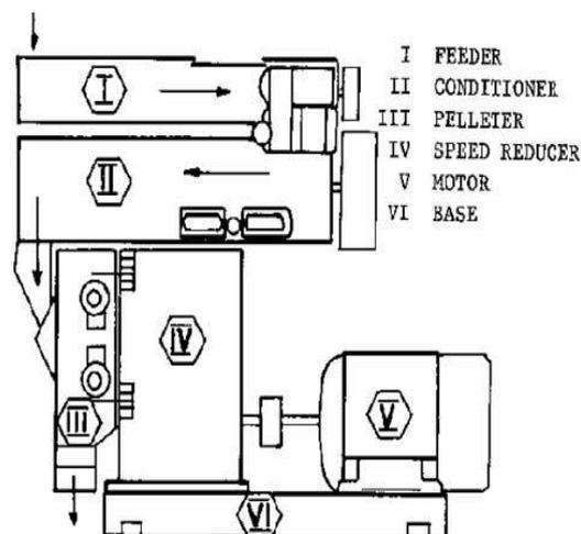
Diagram of Pellet Mill Machines and Parts
