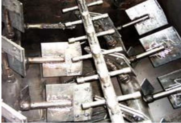
Diagram of a Horizontal Feed Mixer
