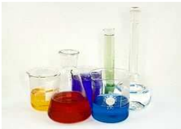
Three beakers, a conical flask, a graduated cylinder and a volumetric flask (Retrieved from " http://en.wikipedia.org/wiki/Laboratory_glassware ")
