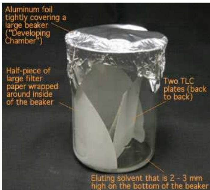
**Plate 2.2: Plate Showing TLC Developing Tank**
