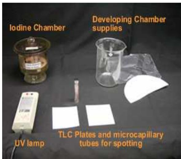
**Plate 2.1: Apparatus required for Thin Layer Chromatography Technique**
