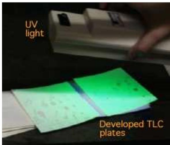
**Plate 2.3: Developed Plate under UV light to see the components as dark spots against a bright green-blue background.**
