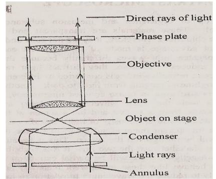
Fig. 2.1: Schematic Illustration of Light Rays in Phase Contrast Microscope
