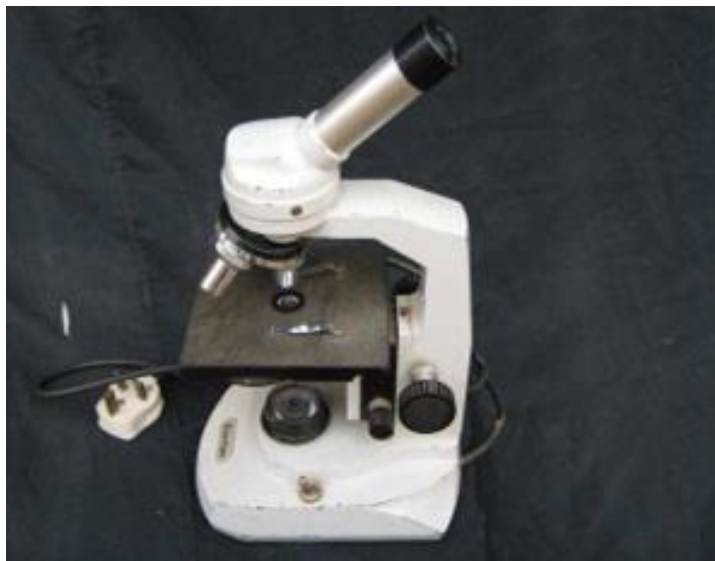
Fig.1.2 Simple compound microscope without condenser lens beneath the stage. (Photo from Bup Oyesiku Bryolab, 2011)
