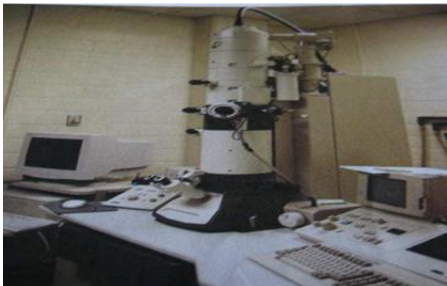
Fig 1.5: Transmission Electron Microscope (TEM)(Photo Bup Oyesiku Bryolab, 2011)
