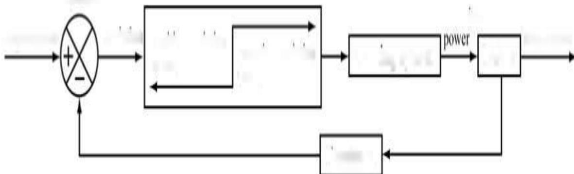
Sometimes, we may use the output of the control system to adjust the input signal. This is called feedback. Feedback is a special feature of a closed loop control system. A closed loop control system compares the output with the expected result or command status, then it takes appropriate control actions to adjust the input signal. Therefore, a closed loop system is always equipped with a sensor, which is used to monitor the output and compare it with the expected result.
