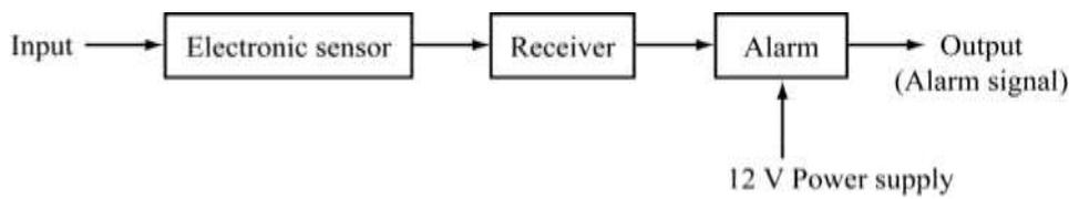
Fig. 13 **Block diagram of an open loop control system (burglar alarm)**
