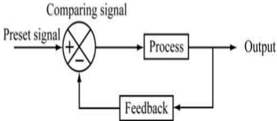
**Fig. 14 Block diagram of a closed loop control system**
