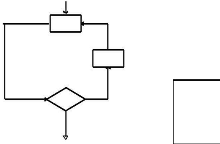
Figure 3: Iteration Construct
