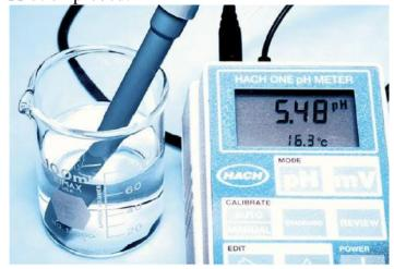
pH meters are used to measure pH values of water samples, such as determining acidity of rainwater samples. Rain water is contains dissolved carbon dioxide that produces a weakly acidic solution. Rain naturally has a pH between 5 and 6. The pH of rain in parts of the U.S. is less than pH 5, which is harmful to aquatic life and human health. This is acid rain.
