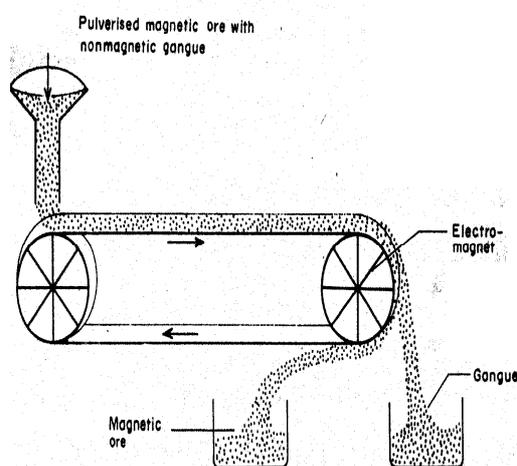
Fig. 5.1: Magnetic separation of ores
