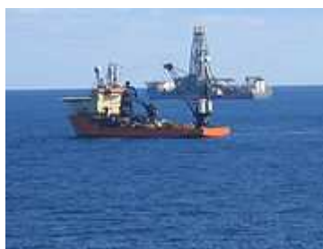
Fig. 2: The Drillship Discoverer Enterprise is shown in the background, at work during exploratory phase of a new offshore field. The Offshore Support Vessel Toisa Perseus is shown in the foreground, illustrating part of the complex logistics of offshore oil and gas exploration and production. (Source: http://www.wikipedia.org )
