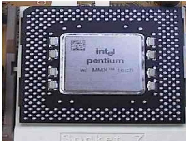
**Fig. 6: An Intel processor**
