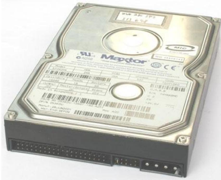
**Fig. 8: The hard drive (Hard disk)**
