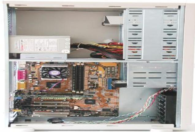
**Fig. 4: Inside the system unit**
