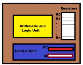
Figure 13: Functional Parts of the Central Processing Unit (CPU) Commented [5]: Here too
