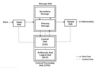
Figure 11: Block Diagram of a Computer
