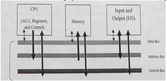
Figure 9 System Bus Model
