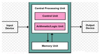
Figure 8: Von Neumann's model of Conventional Digital Computers
