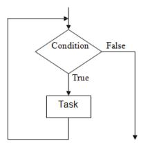
Figure 5: Repetition or Iteration Structure
