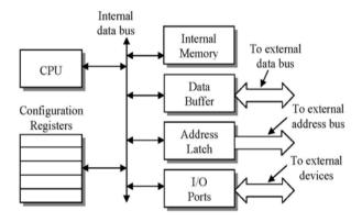
Figure 12: Generic Block Diagram of Processor Internals
