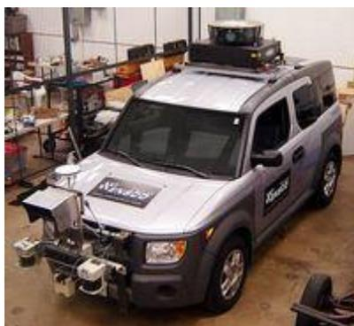
*Figure 9:* RADAR, GPS, LIDAR, ... are all combined to provide proper navigation and obstacle avoidance
