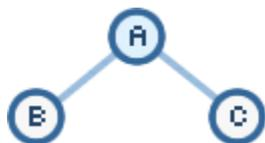
We remove A from our Open list and add A to our Closed List. A's neighbours, the B and C nodes, are added to our Open list. They are added to the end of our Open list, but since our Open list was empty (after removing A), it's hard to show that in this step.
