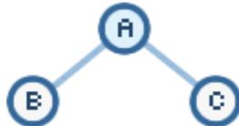
Node A's neighbors are the B and C nodes. Because we are now done with our A node, we can remove it from our Open list and add it to our Closed List. You aren't done with this step though. You now have two new nodes B and C that need exploring. Add those two nodes to our Open list.
