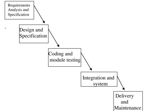
Figure 1.3 : Waterfall Model of Software life Cycle
