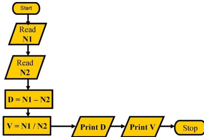
When you draw a flowchart, you should use industry-standard shapes to represent each step in the process. You usually draw the flow from top to bottom or from left to right. Arrows connect the shapes to define the flow. The oval is a terminator and marks the beginning and end of the flow. The parallelograms are used to represent input and output. The rectangles are used to represent a process.
