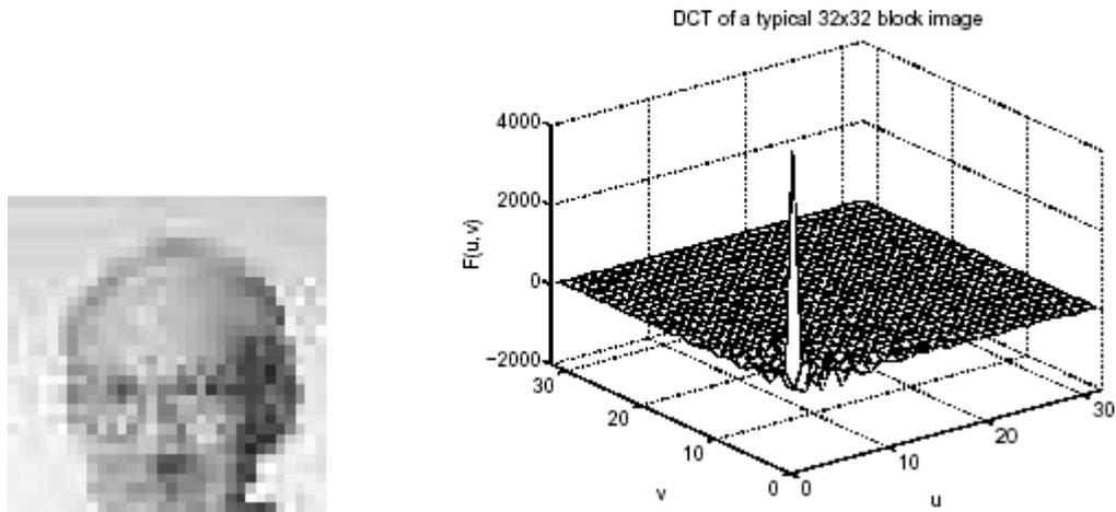
**Fig. 2.3: (a) 32 x 32 pixel version of our standard test image. (b)The DCT of this image.**
