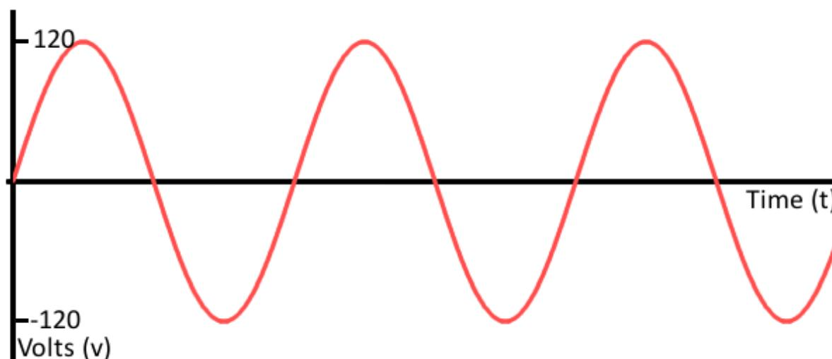
These analog signals must be converted to digital signals that computer can readily deal with using a special hardware devices called *Analog-to-Digital* converters.
