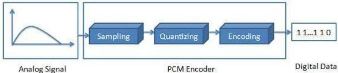
Fig 1: Analog audio signal to digital audio signal
