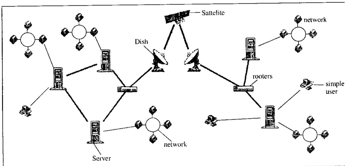
Fig.1.1: *The Physical Components of the Internet*
