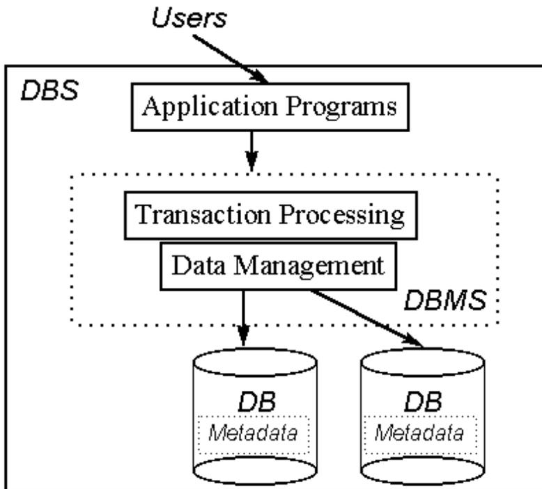
**Figure 1.1** Block diagram of a Database system
