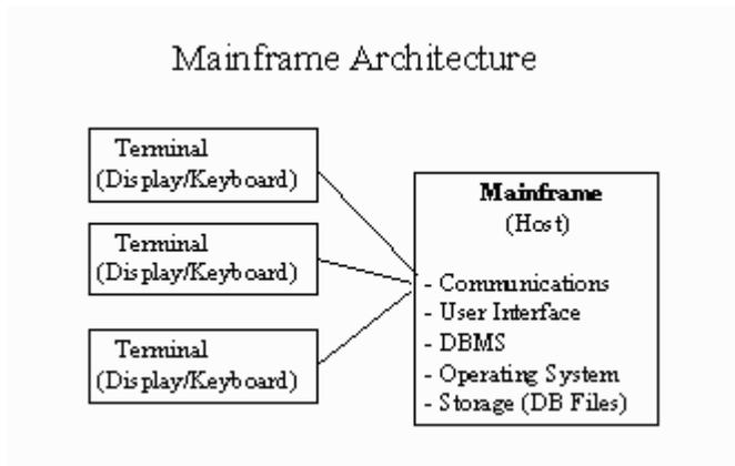
**Figure 11.1 Mainframe Architecture**
