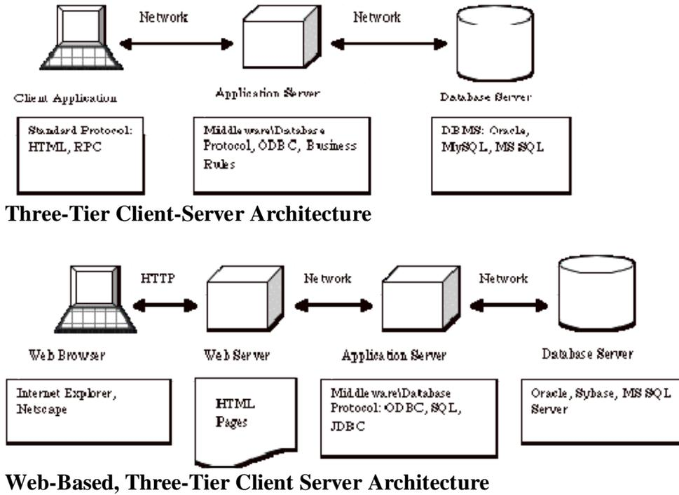
**Figure 11.5 Three-Tier Client/server Architecture**
