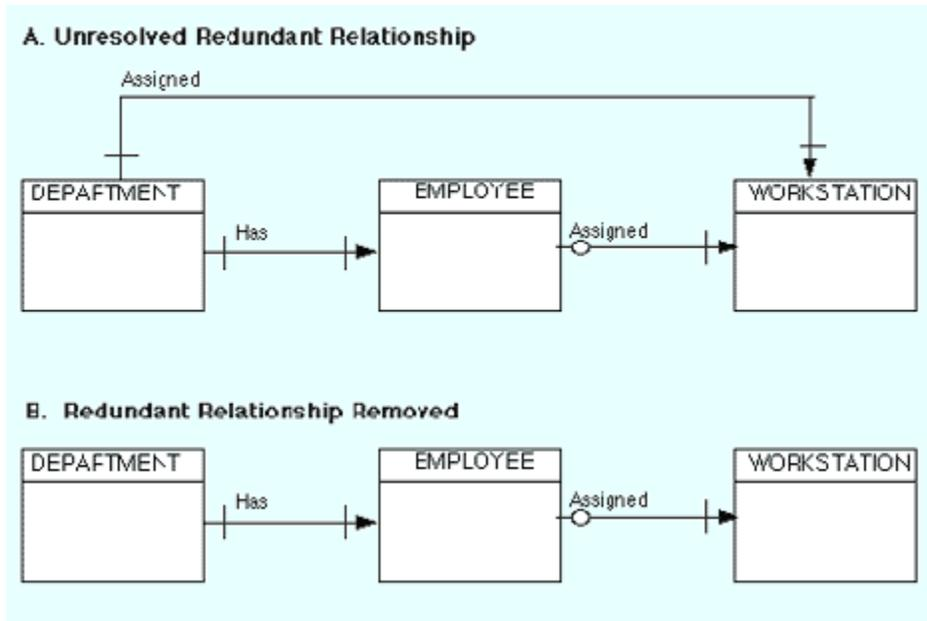
**Figure 3.3: Removing A Redundant Relationship**
