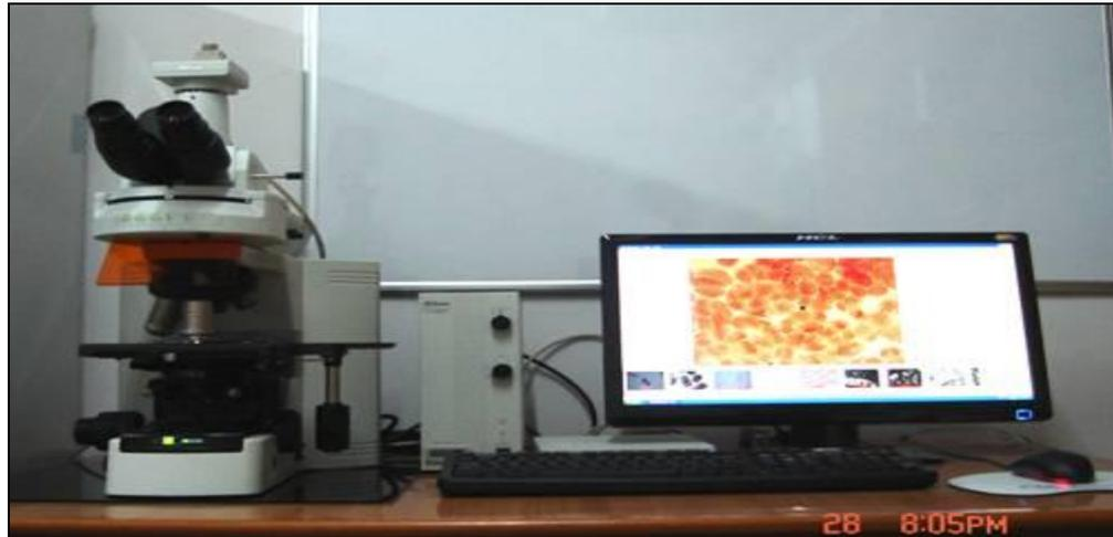
**Figure 5.6:** Upright light microscope with CCD camera attachment
