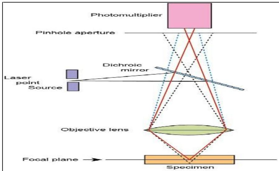
**Figure 2.3:** Confocal principle in epifluorescence laser scanning microscope
