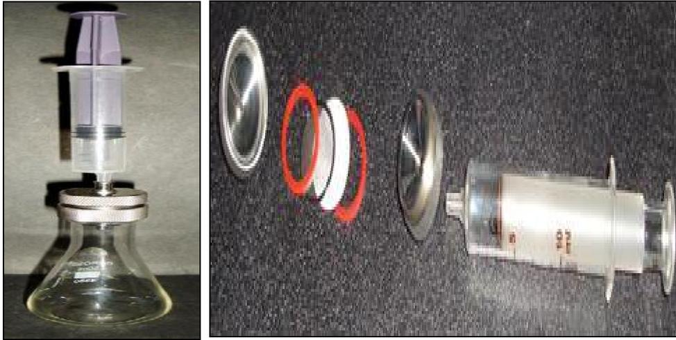
**Figure 5.9: (A) Syringe with filter assembly fitted on conical flask, (B) Disassembled filter assembly**
