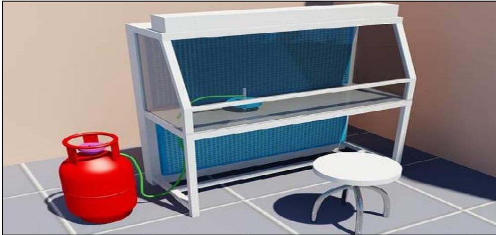
**Figure 5.3:** Laminar-air-hood with coarse filter, HEPA filter, gas cock, gas cylinder and electrical outlets
