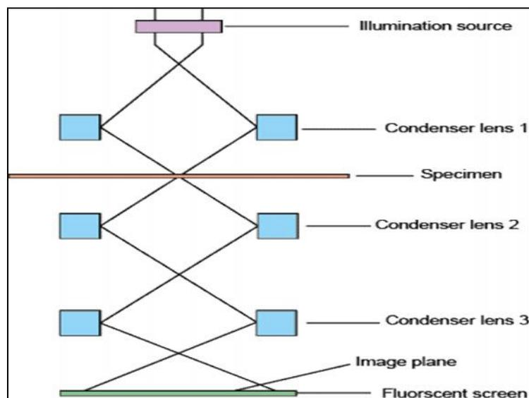
**Figure 3.3:** Organisation of Transmission Electron Microscope
