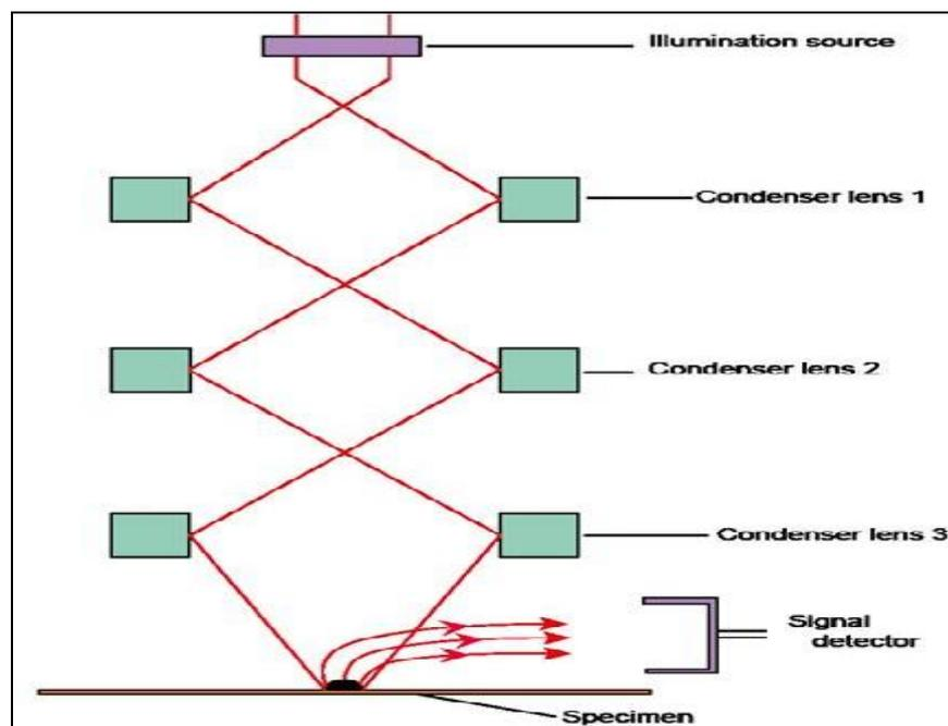
**Figure 3.2:** Configuration of scanning electron microscope
