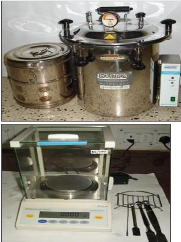
**Figure 5.5:** Autoclave with accessories and High Precision Weighing Balance
