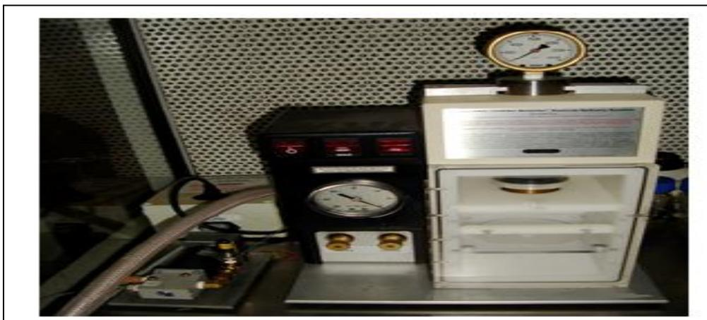
**Figure 2.1:** A gene gun apparatus
