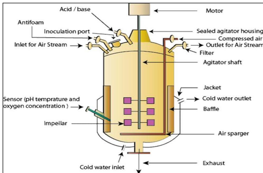
**Figure 5.1:** Diagram of a typical bioreactor.
