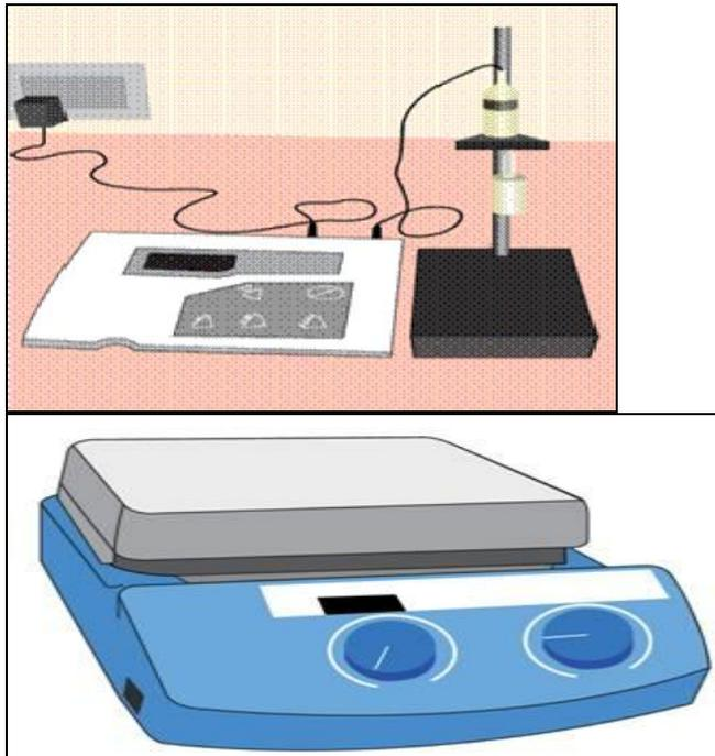
**Figure 5.4:** pH Meter and Magnetic stirrer-cum-heater
