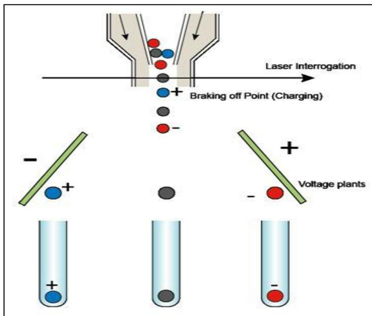
**Figure 4.1:** Electrostatic flow sorting
