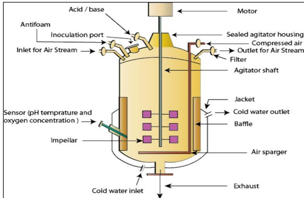
**Figure 5.1:** Diagram of a typical bioreactor.
