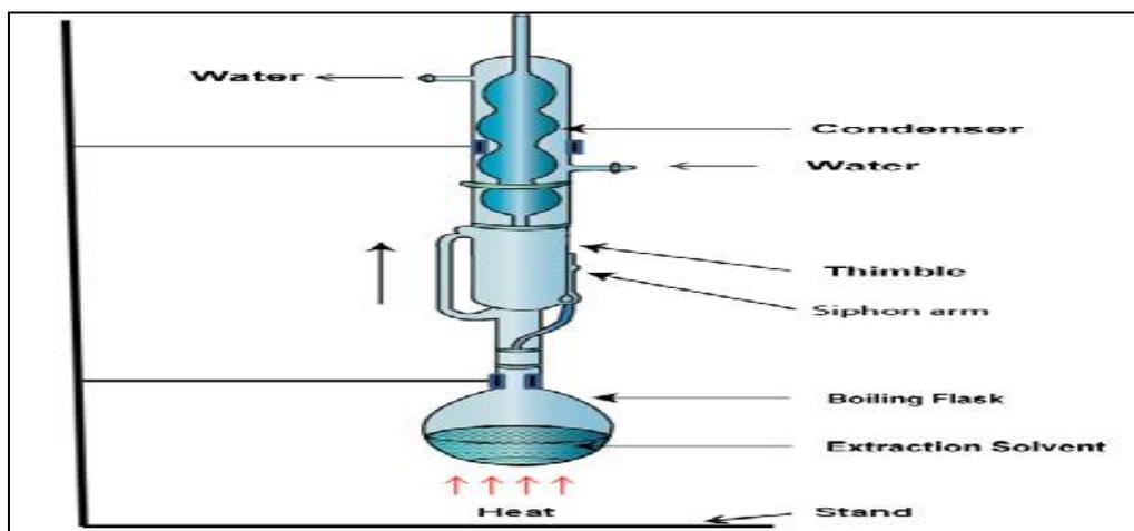
**Figure 2.1:** A Soxhlet apparatus
