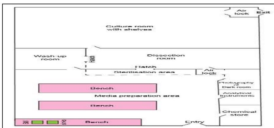
**Figure 5.1:** A floor plan for plant tissue culture laboratory
