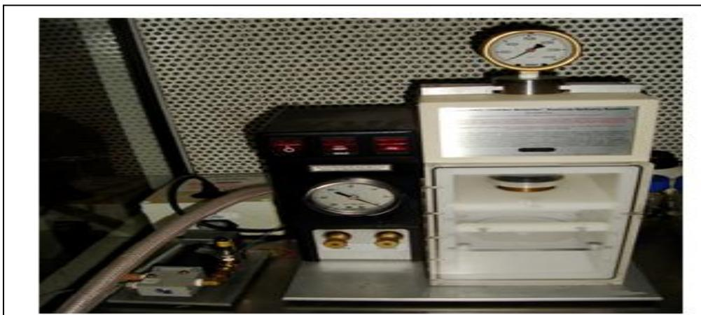
**Figure 2.1:** A gene gun apparatus
