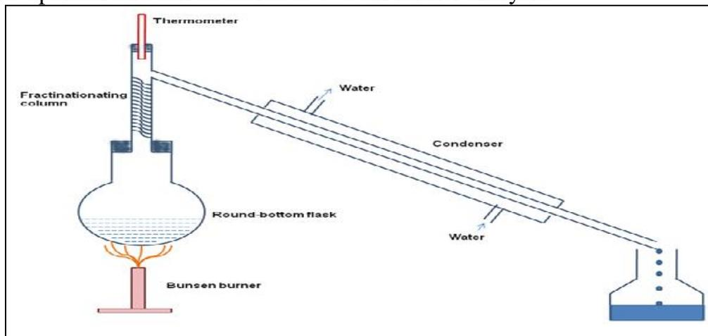
**Figure 3.1:** A simple fraction distillation apparatus
