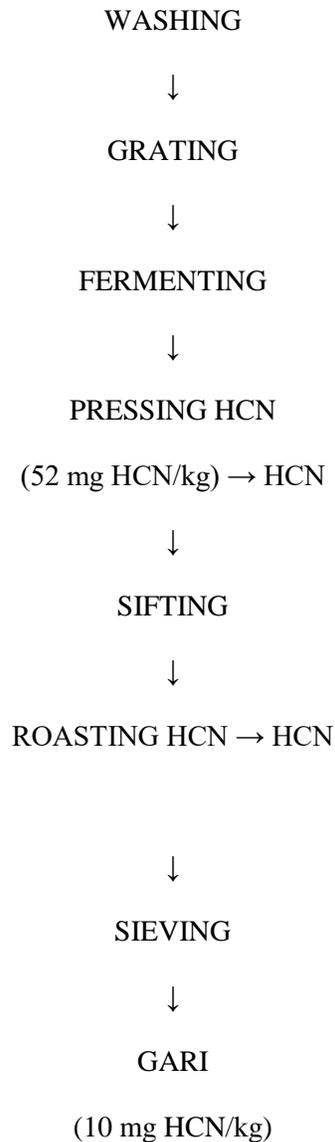
Figure 1: Process flow chart for gari production
