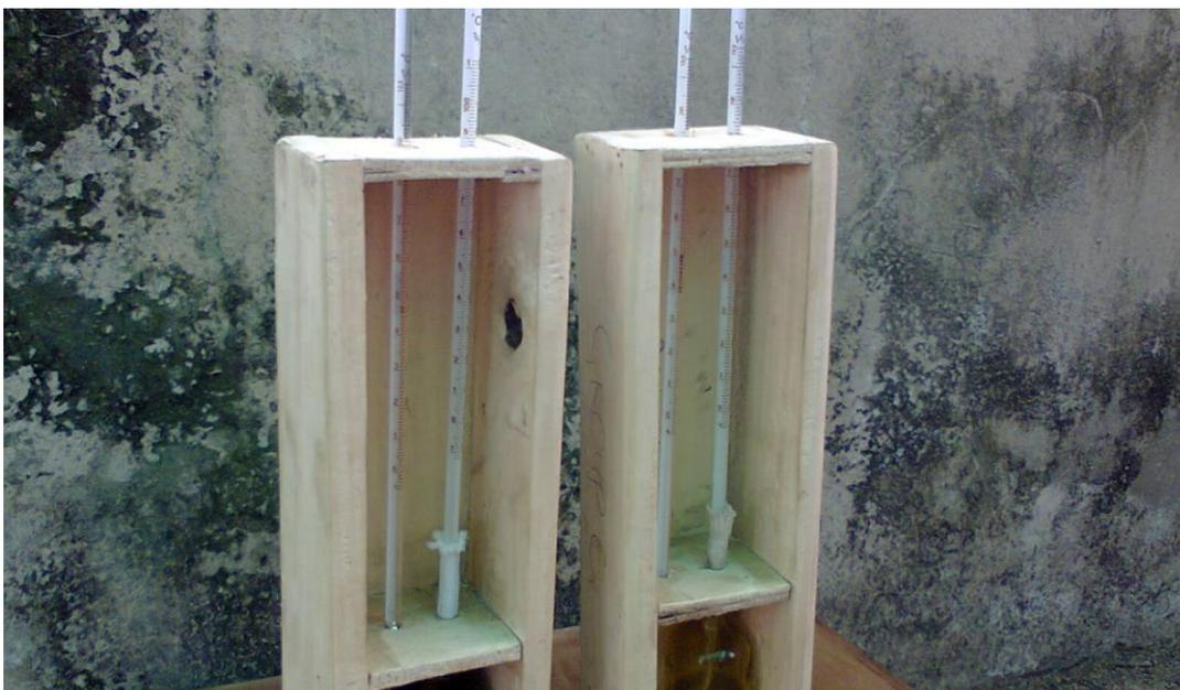
**Figure . Locally constructed Hygrometer**
