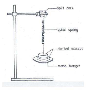
You have been provided with a retort stand, clamp and boss, a set of masses, a spiral spring, stop watch, split cork and other necessary apparatus.
