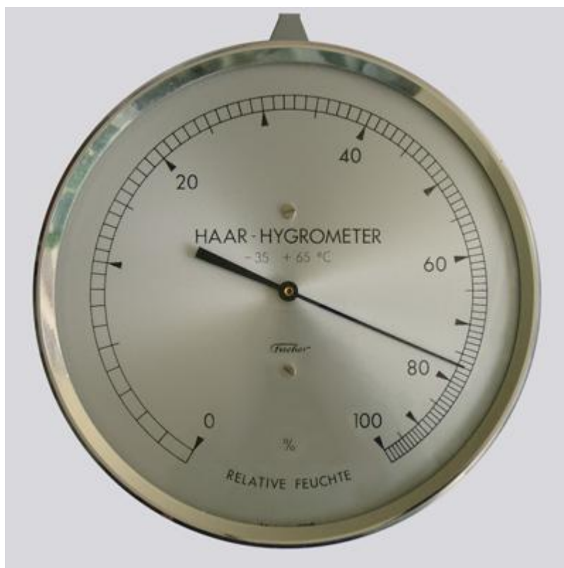
Fig. 1.3: A Typical Haar Hygrometer
