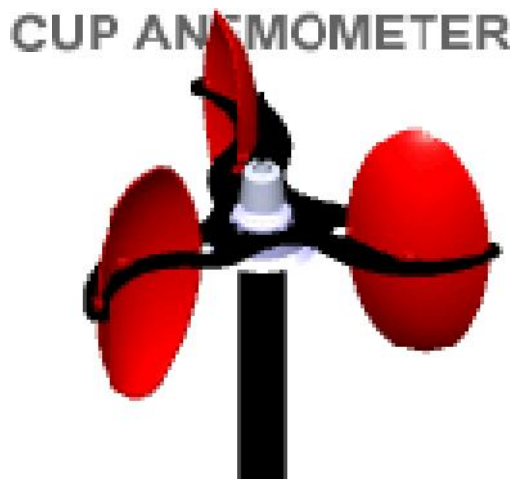
Fig. 1.5: A Three Cup Anemometer
