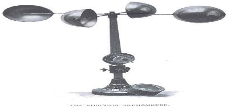
Fig. 1.6: A Typical Four Cup Anemometer
