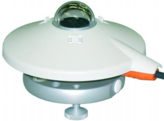
Fig. 1.1: A Typical Glassed Dome Pyranometer
