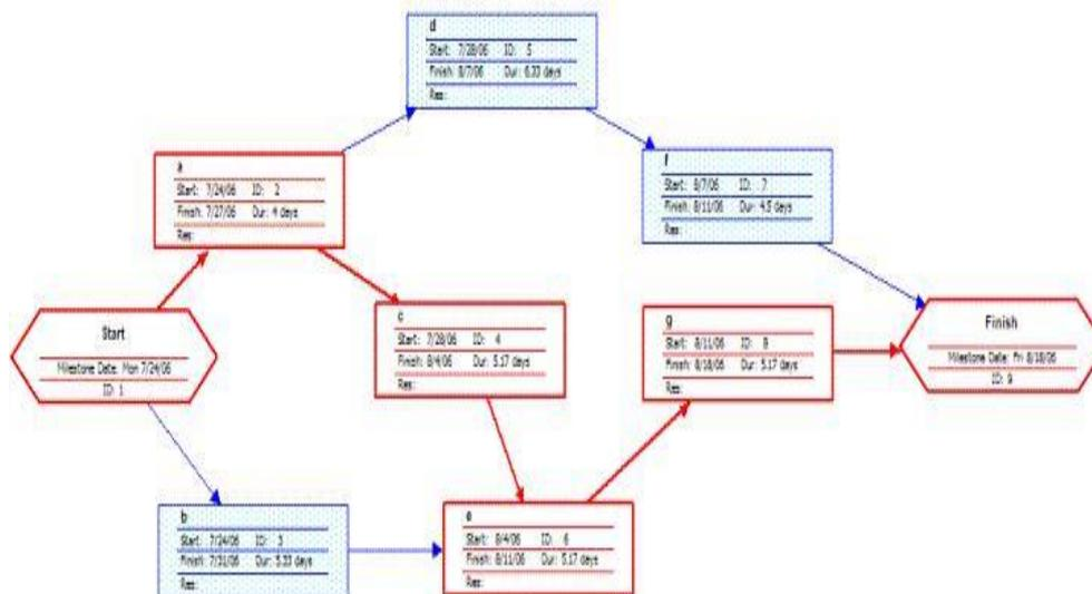
**A network diagram created using Microsoft Project (MSP). Note the critical path is in red.**
