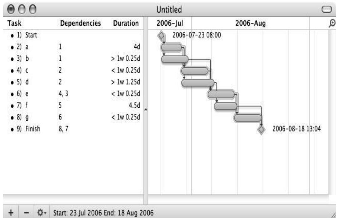
A Gantt chart created using OmniPlan. Note (1) the critical path is highlighted, (2) the slack is not specifically indicated on task 5 (d), though it can be observed on tasks 3 and 7 (b and f), (3) when using OmniPlan, you may use the GUI to easily link dependencies, or you may enter them by reference to task ID, and (4) since weekends are indicated by a thin vertical line, and take up no additional space on the
