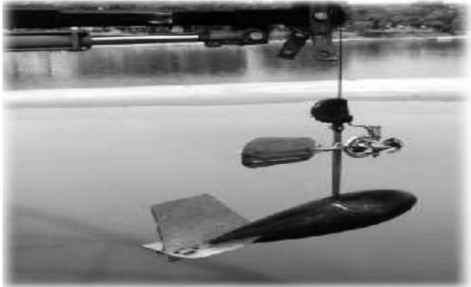
Fig. 11.3: A current meter inserted into the stream
