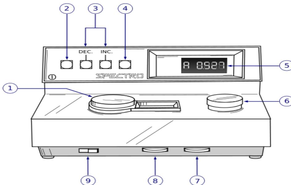
**Fig 2.3:** A typical colorimeter
