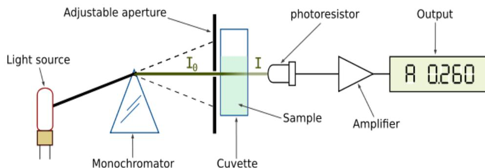
**Fig. 5.2:** Composition of a typical colorimeter
