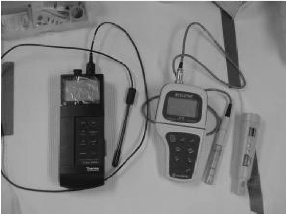
These three meters and probes can measure pH (left) and electrical conductivity (center and right)
