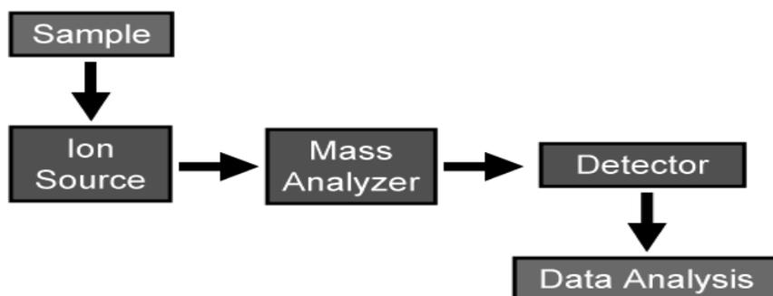
**Fig. 5.3:** an operational scheme of a Mass Spectrometer
