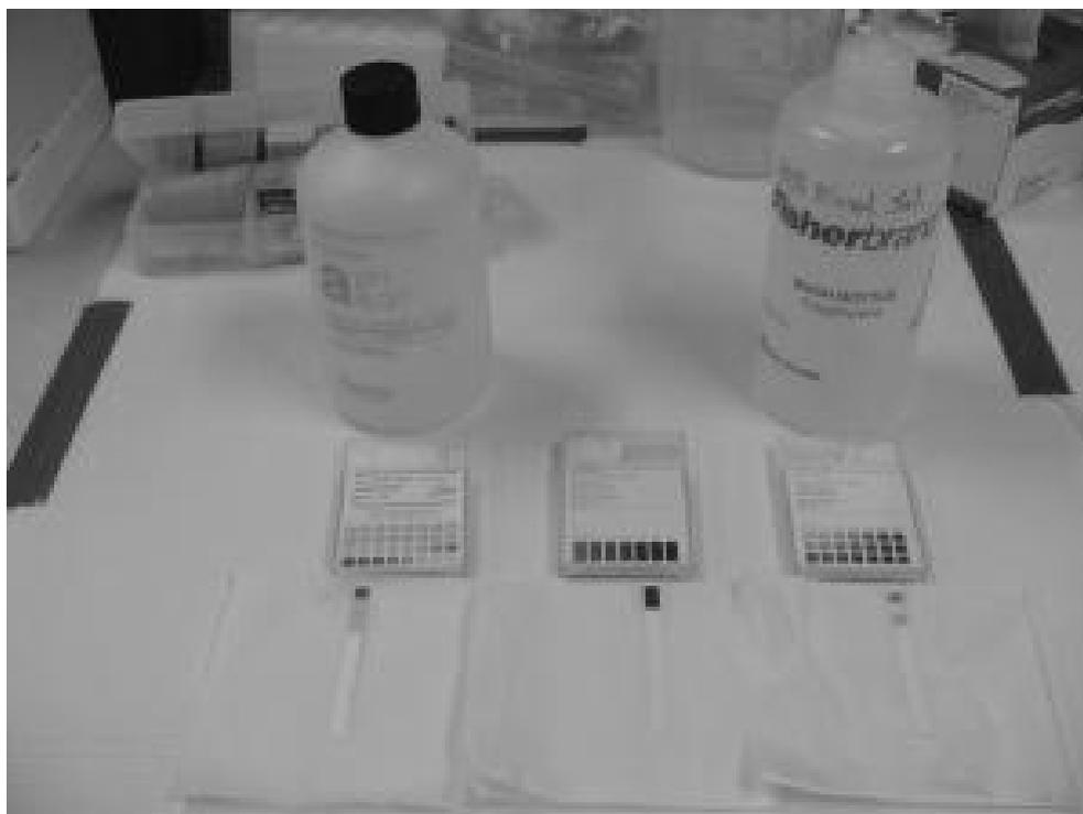
These pH strips can measure pH in a series of ranges by putting sample on a strip and comparing its colour change with colors on the box that correspond to a certain pH. The strip on the left measures pH 0-7 and shows results of a strong acid sample; the center strip is pH range 5-10 and shows results of a 6.97 buffer solution sample; the strip on the right measures a broad range (pH 1-14) and shows results of a 10% bleach water solution sample.
