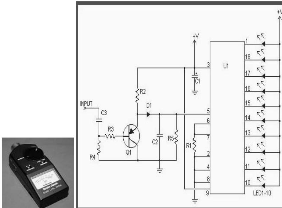
**Electric circuit of a sound meter**
