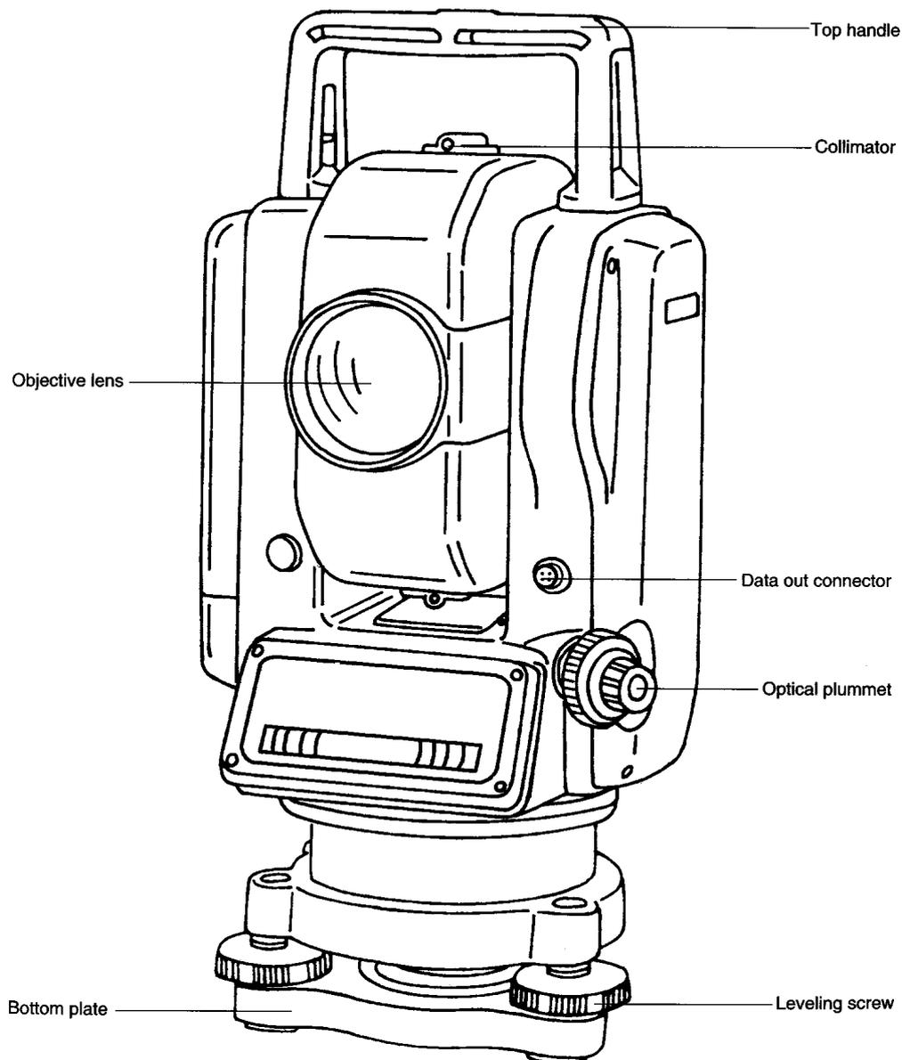
**Fig. 2.4:** Image of a Total station
