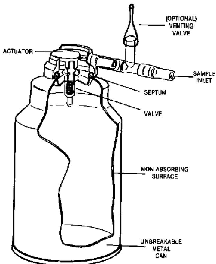
**Fig. 6.1:** A typical steel evacuated sampler
