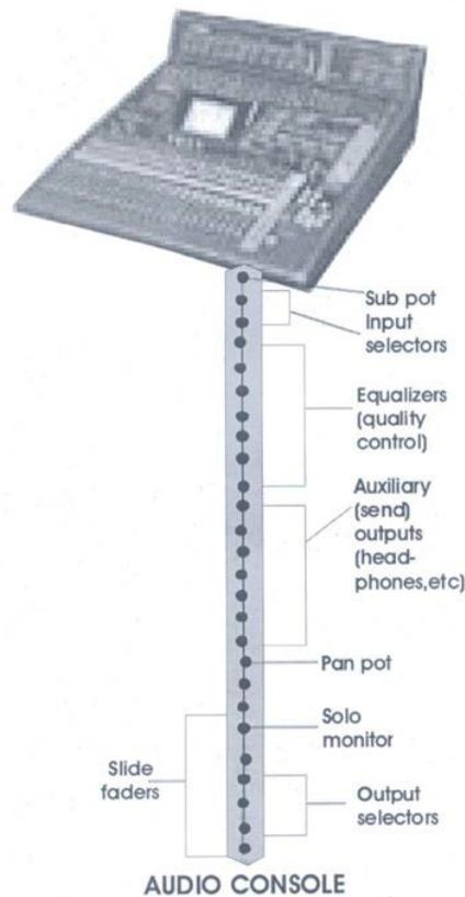
**Mix:** The audio console enables one to combine, or mix, the signals from various inputs, such as two lavalier mics, background music, and the sound effect of a phone ring. The mix bus combines (mixes) these various audio signals with the specific volume assigned by the operators. Without the mixing capability of the board, one could control only one input at a time. The completed mix is then fed to the line-out.
