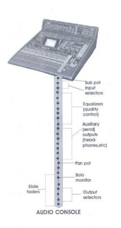
**Mix:** The audio console enables one to combine, or mix, the signals from various inputs, such as two lavaliere mics, background music, and the sound effect of a phone ring. The mix bus combines (mixes) these various audio signals with the specific volume assigned by the operators. Without the mixing capability of the board, one could control only one input at a time. The completed mix is then fed to the line-out.
