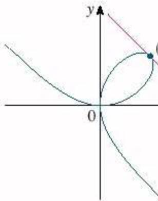
We can see in a plot of the implicit function that the slope of the tangent line at the point (3,3) does appear to be -1.
