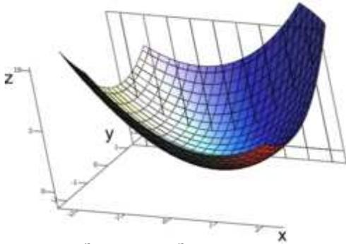
A graph of  $z = x^2 + xy + y^2$ . For the partial derivative at  $(1, 1, 3)$  that leaves  $y$  constant, the corresponding tangent line is parallel to the  $xz$ -plane.
