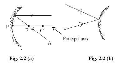
Because the convex mirror or the concave mirror is part of a sphere, it has a center C called the center of curvature, and a radius (r) called radius of curvature. And it also has a Principal Focus F<sub>1</sub>, whose distance from the pole P to the mirror is half the radius of curvature. These parameters are shown in Fig. 2.2 for the convex mirror respectively.
