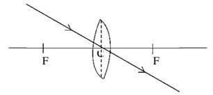
Fig. 5.1 (c): A ray incident along the optical centre of the line is undeviated and passes to the other side without any deviation.
