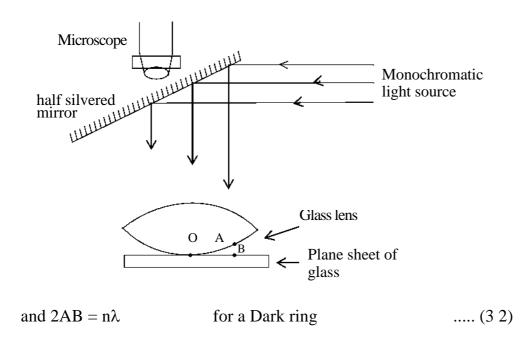
Fig. 3.1: Newton's rings experiment arrangement
