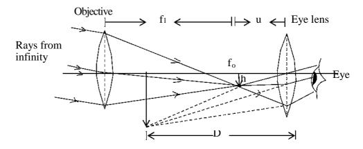
Fig. 5.2: Telescope with image formed at near point.
