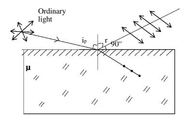
Fig. 5.1: Polarization by reflection
