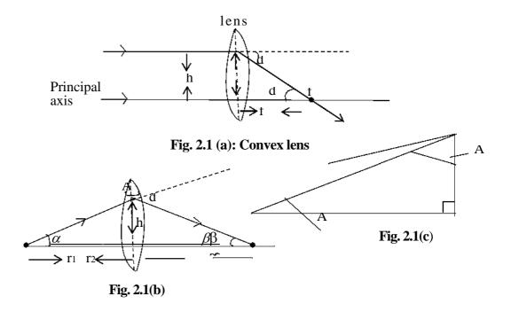
When a ray of light enters a prism, it deviates. Let d be the angle of deviation of light from a small angle prism. The small angle of the prism is A. Let  $\mu$  is the refractive index of the glass. Then the expression for the deviation of a ray passing through a prism can be written as
