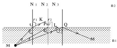
Fig. 3.4: When light travels from water to air, the angle of incidence i2 produce the angle of refraction of  $90^{\circ}$  ( $r_2 = 90^{\circ}$ ) is called critical angle,  $\theta_c$  ( $i_2 = \theta_c$ ).
