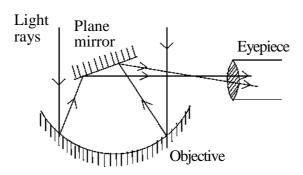
Fig. 5.4: Newton Reflector Telescope
