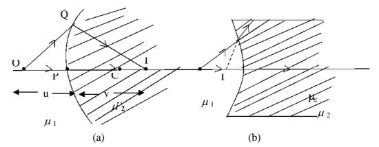
Fig. 5.1: Refraction at curved surface
