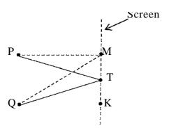
Fig. 1.1: Point of constructive interference (T) and destructive interference (M).
