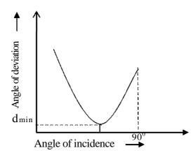
Fig. 4.3: Variation of angle of deviation d with angle of incidence i1
