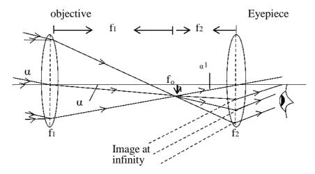
Fig. 4.5: An Astronomical Telescope in normal adjustment.
