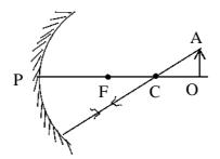
Fig. 2.3 (b): A ray goes through centre of curvature reflected back along its path
