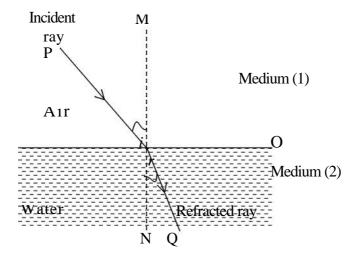
Fig. 3.2: Refraction at plane surface between two medium
