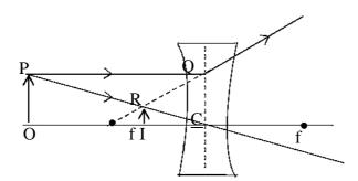
Fig. 5.6: Image formed by a concave lens.
