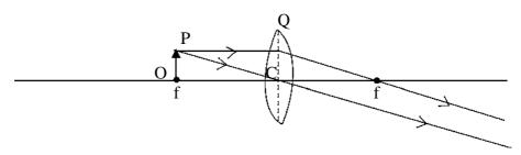
Fig. 5.4: A ray diagram for an object placed at f.
