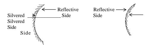
Fig. 2.1 (a) concave mirror (b) convex mirror
