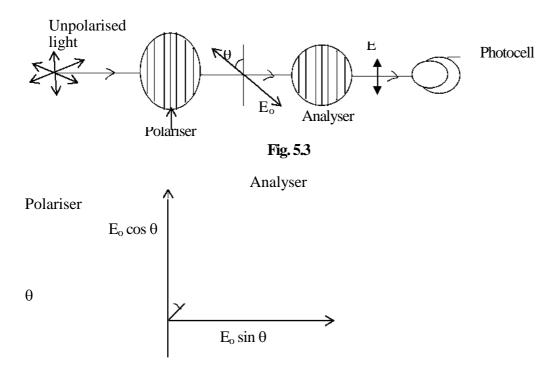
Fig. 5.4: Two components of polarized light.
