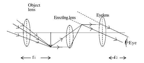
Fig. 5.3: A terrestrial telescope
