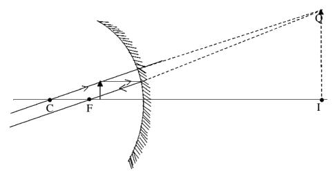
Fig. 2.6: Image formed by a concave mirror for object between F and the mirror.
