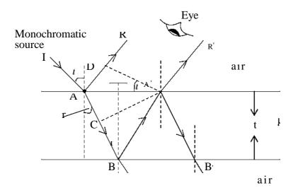
Fig. 3.3: Interference in thin film
