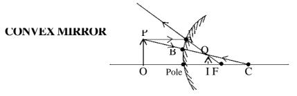
Fig. 2.7: Formation of an image by convex mirror
