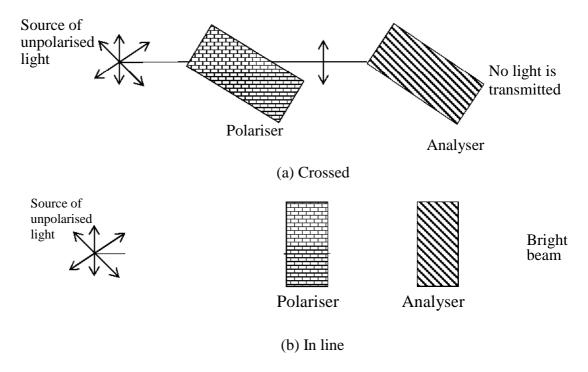
Fig. 4.1: Plane polarization of light
