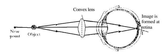
Fig. 3.2 (b): Use of convex lens to correct far sightedness.
