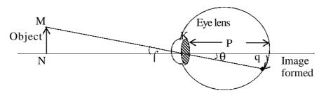
Fig. 4.1: Size of the image on retina, q and angle  $\theta$  subtended on eye.
