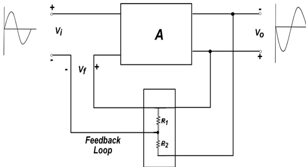
Figure 3.4 - Shunt-derived Series-fed Voltage Feedback
