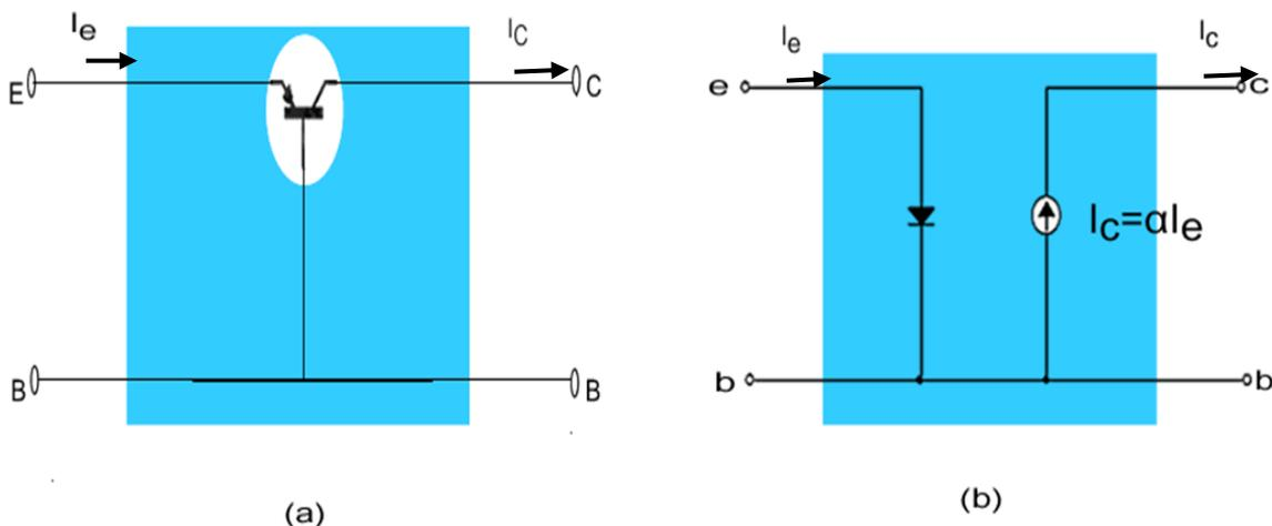
Fig 3.18 (a) Common-base BJT transistor; (b)  $r_e$  model for the configuration
