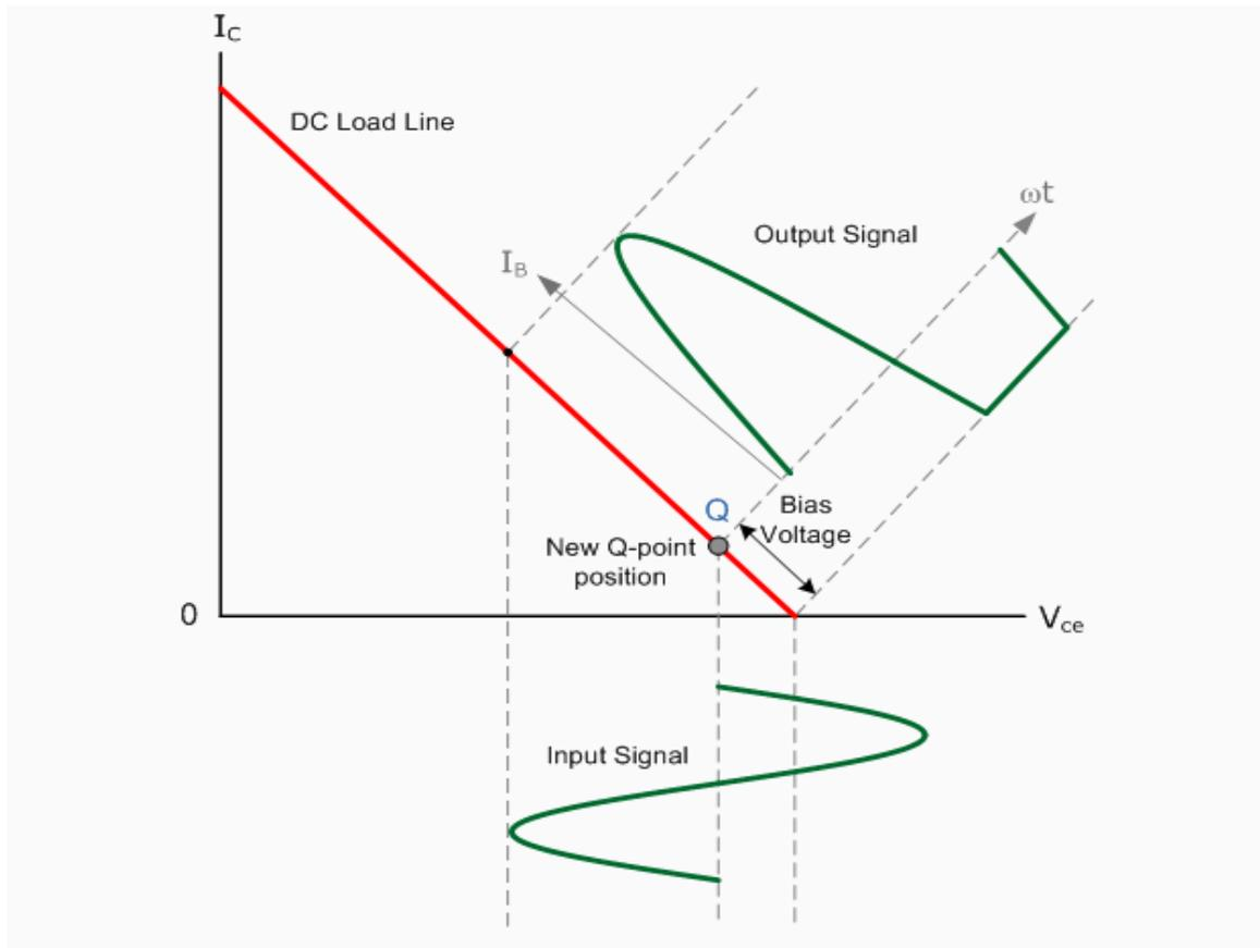
Fig 3.21 Class AB Output Characteristics
