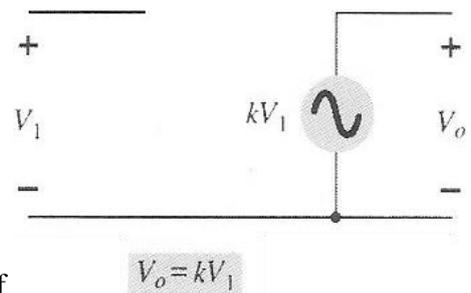
Figure 3.10 Ideal voltage-controlled voltage source.
