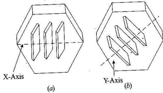
crystal wafers are cut from the crude quartz in two different ways. The method of 'cutting' determines the crystal's natural resonant frequency and its temperature coefficient. When the wafer is cut so that its flat surface is perpendicular to its electrical axis, it is called an X-cut crystal. But if the wafer is so cut that its flat surfaces are perpendicular to its mechanical axis, it is called Y-cut crystal.
