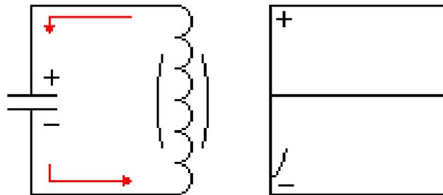
Technically this basic LC circuit generates a sine wave that loses voltage in every cycle. To overcome this, additional voltage is applied to keep the oscillator from losing voltage. However, to keep this oscillator going well, a switching method is used. A vacuum tube (or a solid-state equivalent such as a FET) is used to keep this LC circuit oscillating. The advantage of using a vacuum tube is that they can oscillate at specified frequencies such as a thousand cycles per second.
