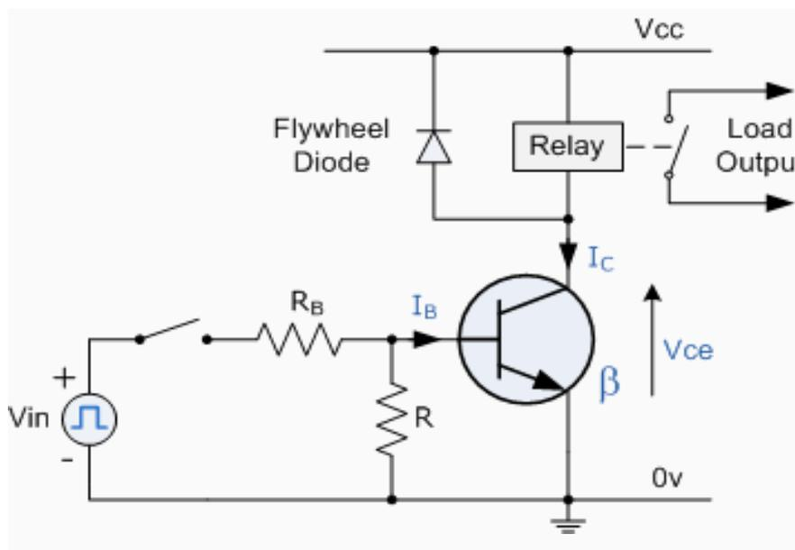
FIG 3.11 Transistor Switching Circuit
