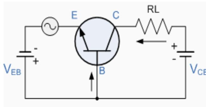
Fig 3.2 the Common Base Amplifier Circuit
