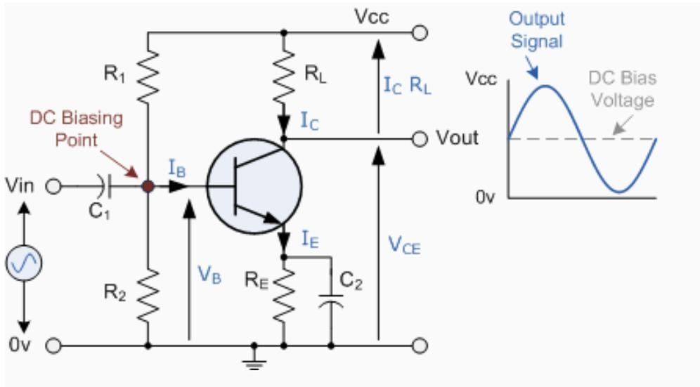
Fig 3.6 the Common Emitter Amplifier Circuit
