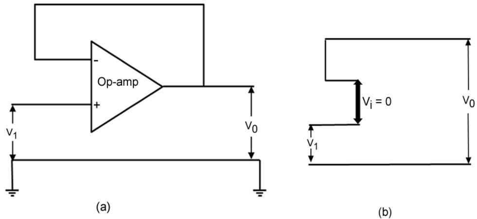
Figure 3.12 (a) Unity follower, (b) virtual-ground equivalent circuit
