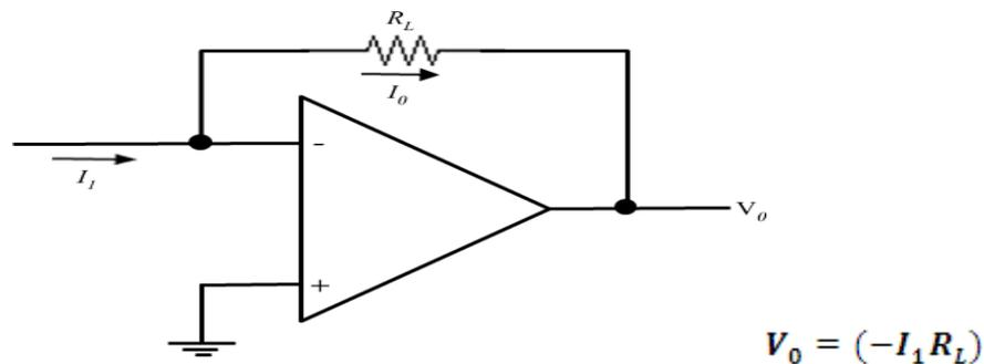
Fig 3.14 Practical form of current-controlled voltage source.
