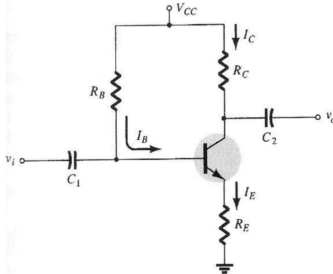
Fig 3.6 BJT bias circuit with emitter resistor.
