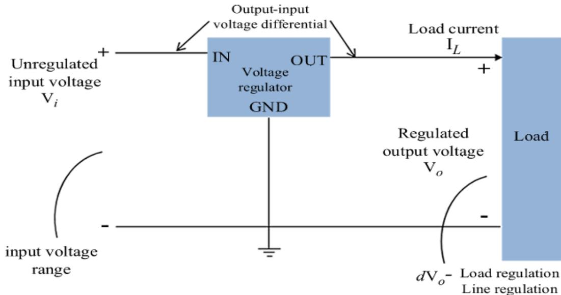
Figure 3.1 Block representation of three terminal voltage regulator
