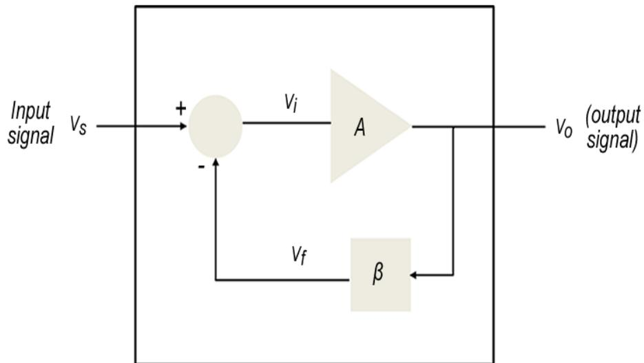
Figure 1.1- Simple block diagram of a feedback amplifier
