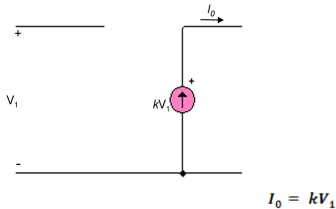
Fig 3.12 Ideal voltage-controlled current source.
