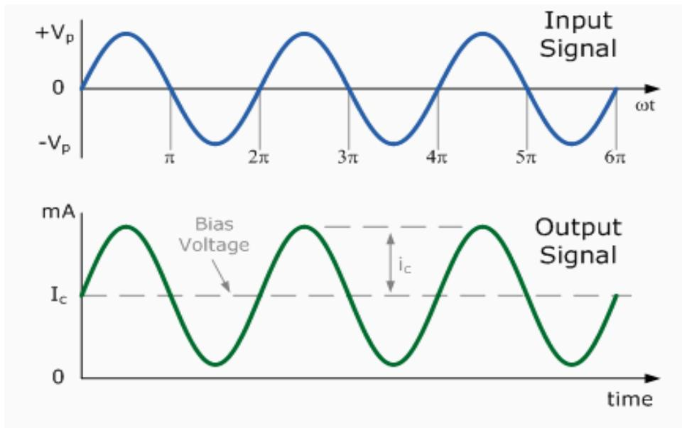
Fig 3.6 Class A Output Waveform
