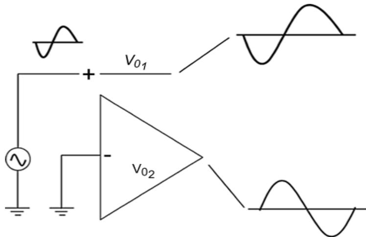
Fig 3.5 Double-ended output with single ended input
