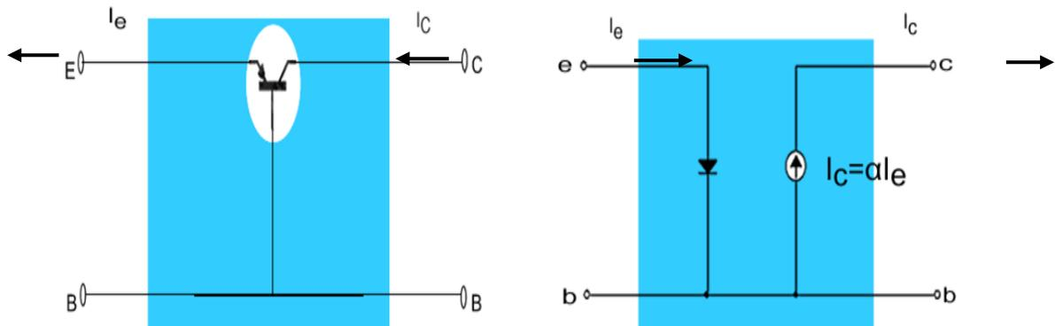
Fig 3.22 Approximate model for a common-base npn transistor configuration
