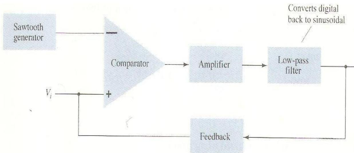
Fig 3.23 Block diagram of class D amplifier.
