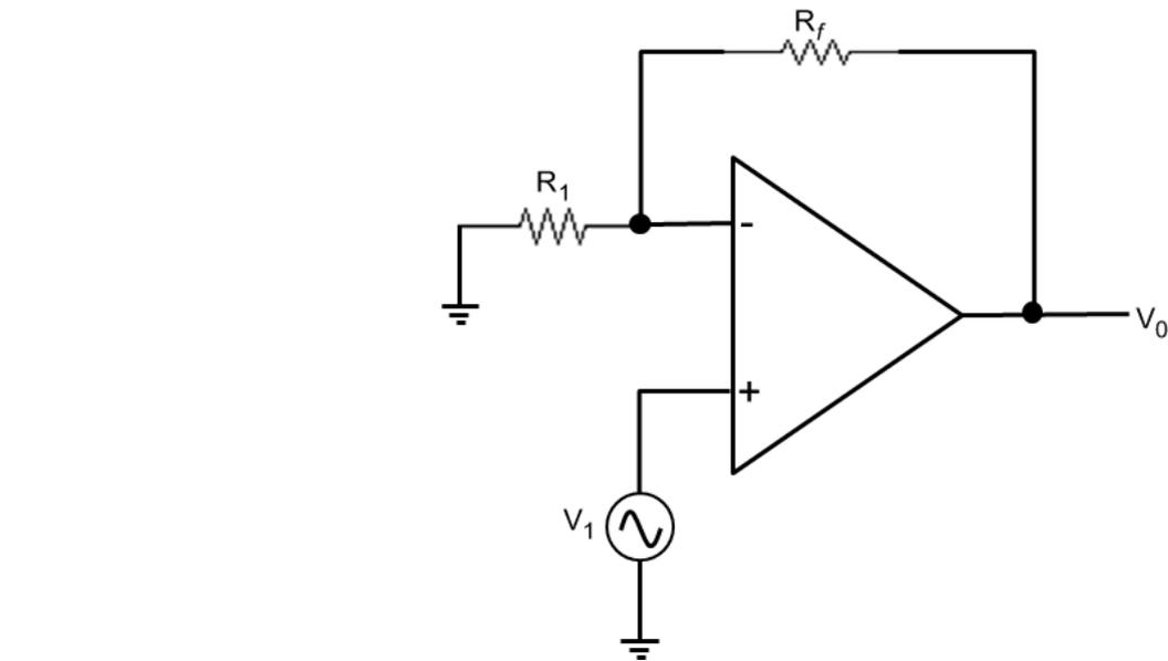
Figure 3.2 Noninverting fixed-gain amplifier.
