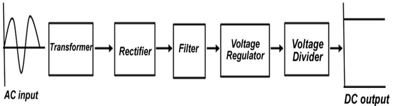
Fig 3.1 dc power supply unit
