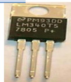
about 22 V, with ac ripple of a few volts as the input to the voltage regulator. The 7812 IC then provides an output that is a regulated +12 V dc.
