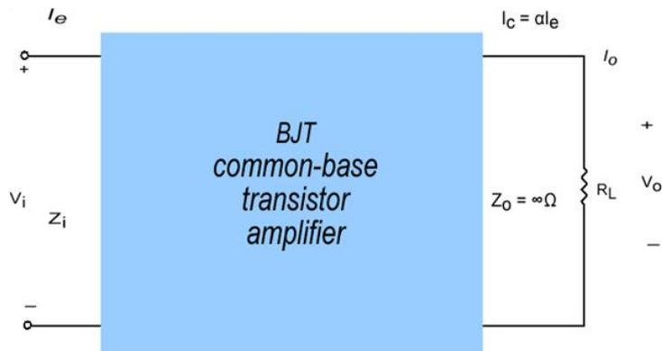
Fig 3.21 Defining  $A_v = V_o/V_i$  for the common-base configuration
