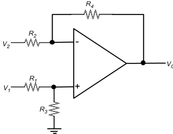
Fig 3.6 Subtraction circuit.
