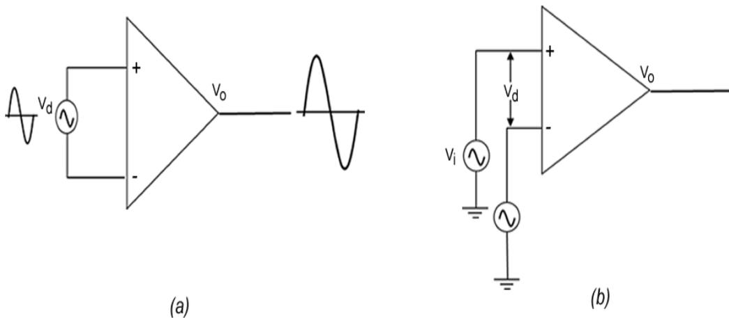
Fig 3.3 Double-ended (differential) operation
