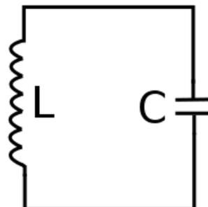
An LC circuit can store electrical energy vibrating at its resonant frequency. A capacitor stores energy in the electric field between its plates, depending on the voltage across it, and an inductor stores energy in its magnetic field, depending on the current through it.
