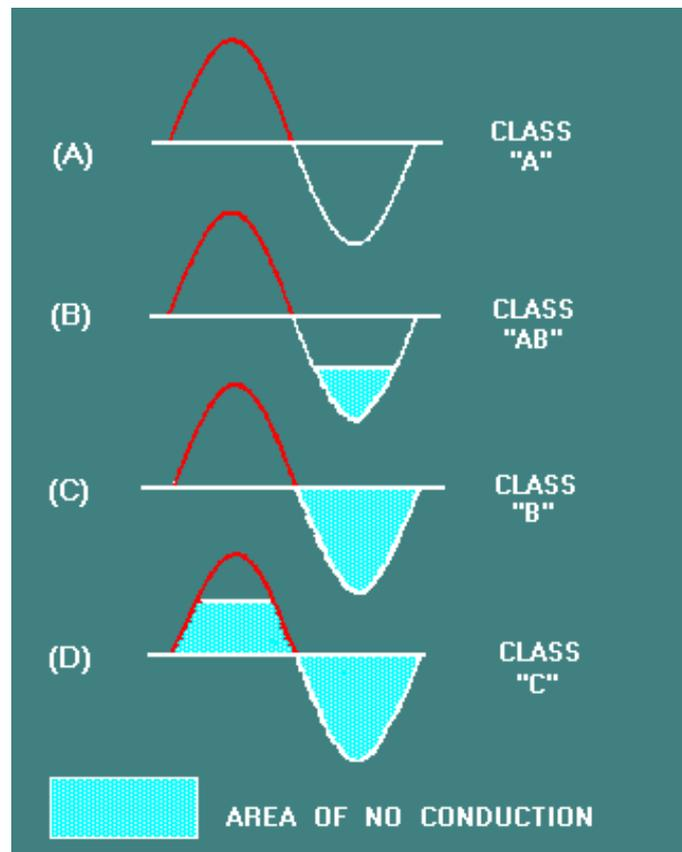
Figure 3.4: comparison of output signals for the different amplifier classes of operation.
