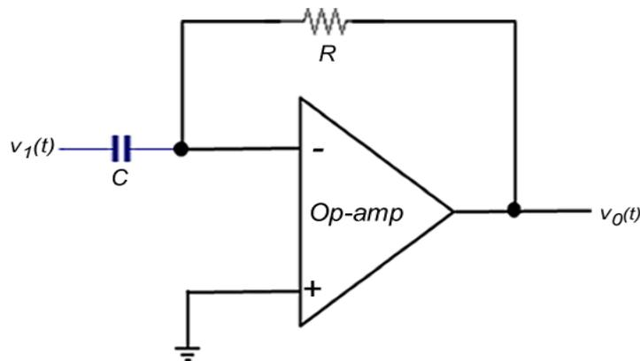
Figure 3.15 Differentiator circuit.
