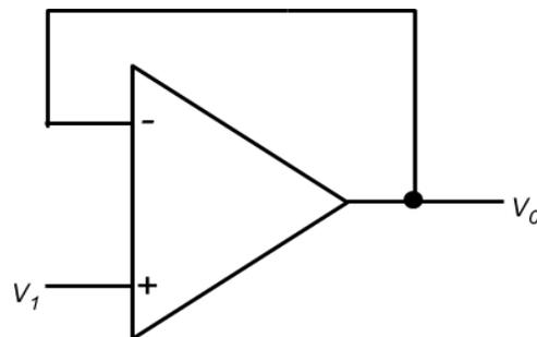
Fig 3.8 Unity-gain (buffer) amplifier
