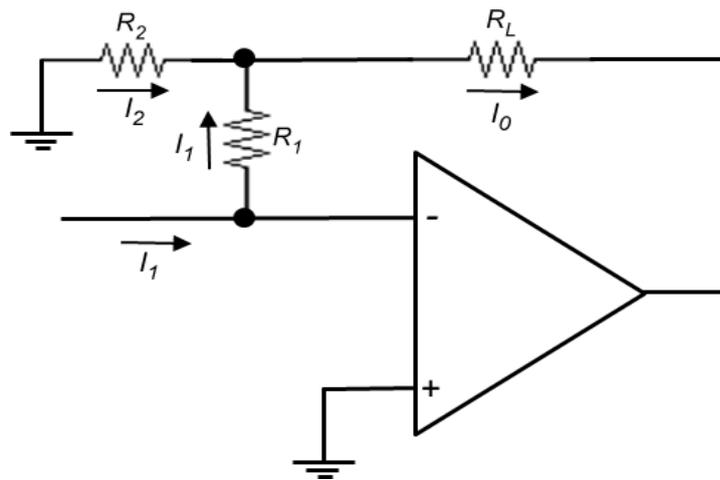
Fig 3.16 Practical form of current-controlled current source
