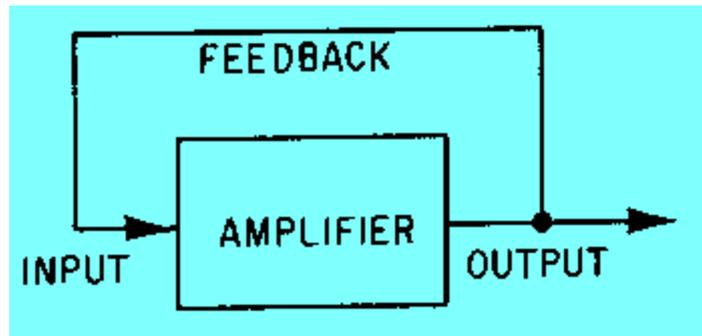
Figure 1.2 - Basic oscillator block diagram.
