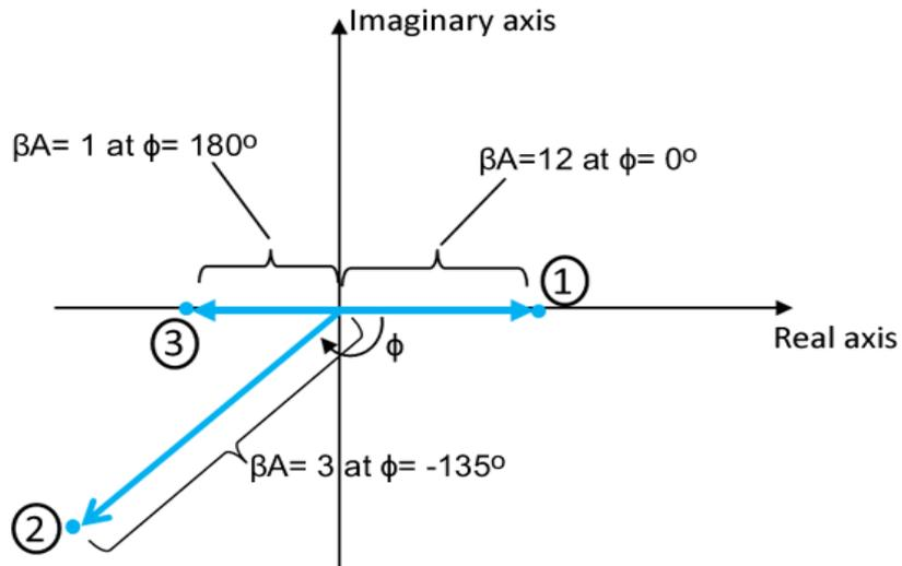
Fig 3.1 Complex plane showing typical gain-phase points.
