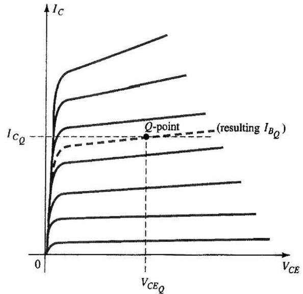
Figure 3.10 Defining the Q-point for the voltage-divider bias configuration.
