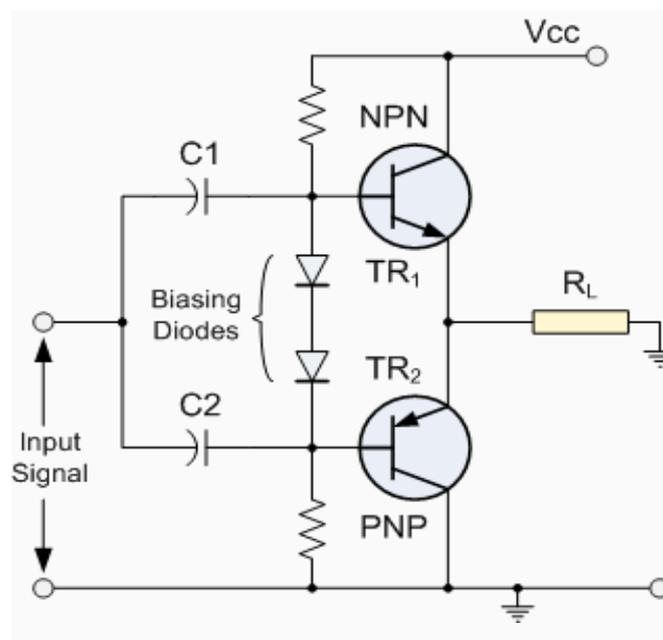
Fig3.20 Pre-biasing with Diodes
