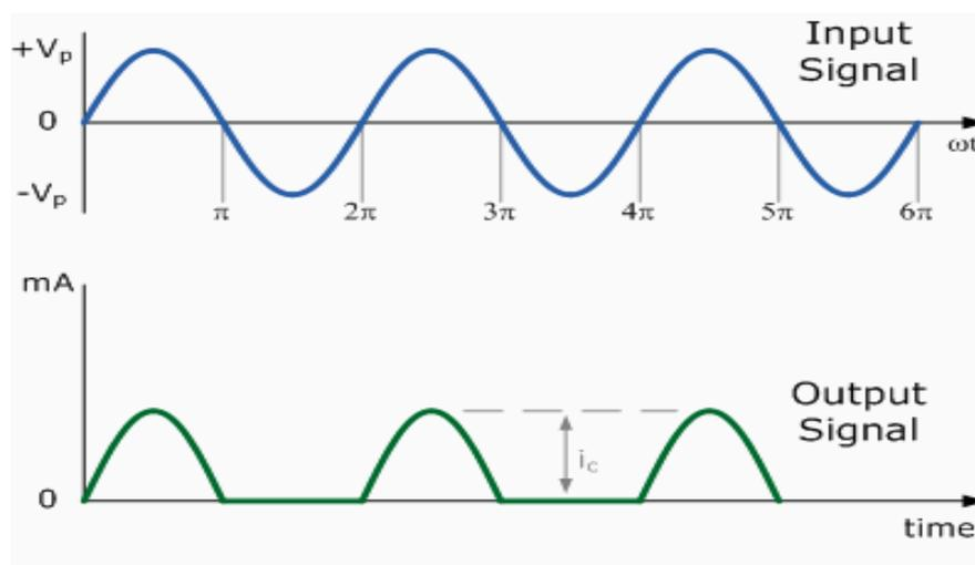
Fig3.11 Class B Output Waveform
