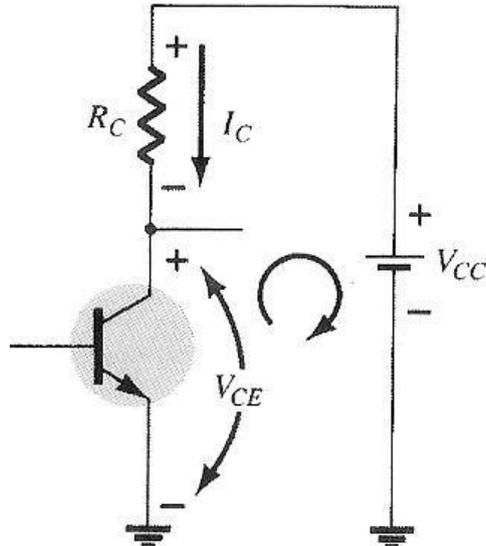
Fig 3.4 Collector-emitter loop.
