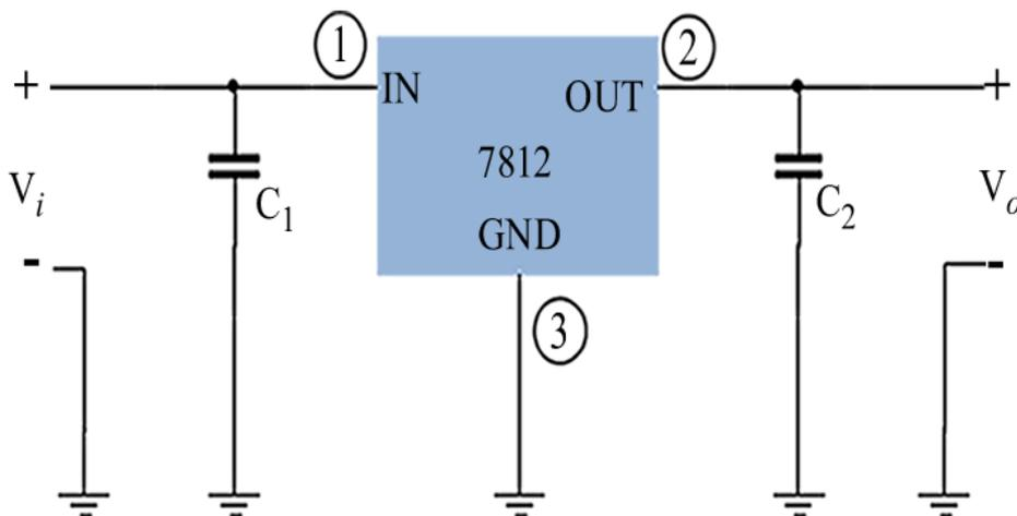
Figure 3.2 Connection of 7812 voltage regulator.
