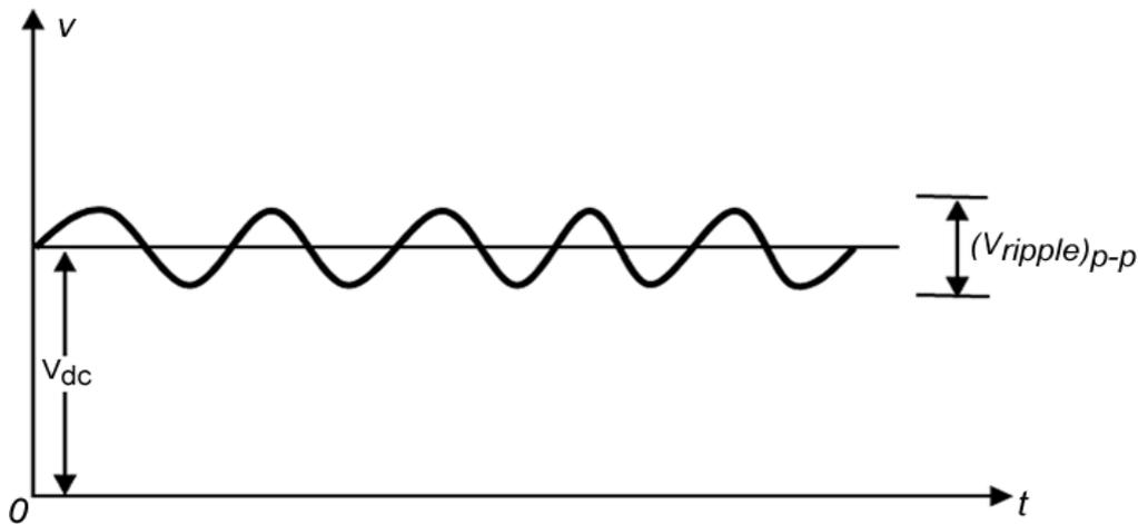
Figure 1.1 Filter voltage waveform showing dc and ripple voltages
