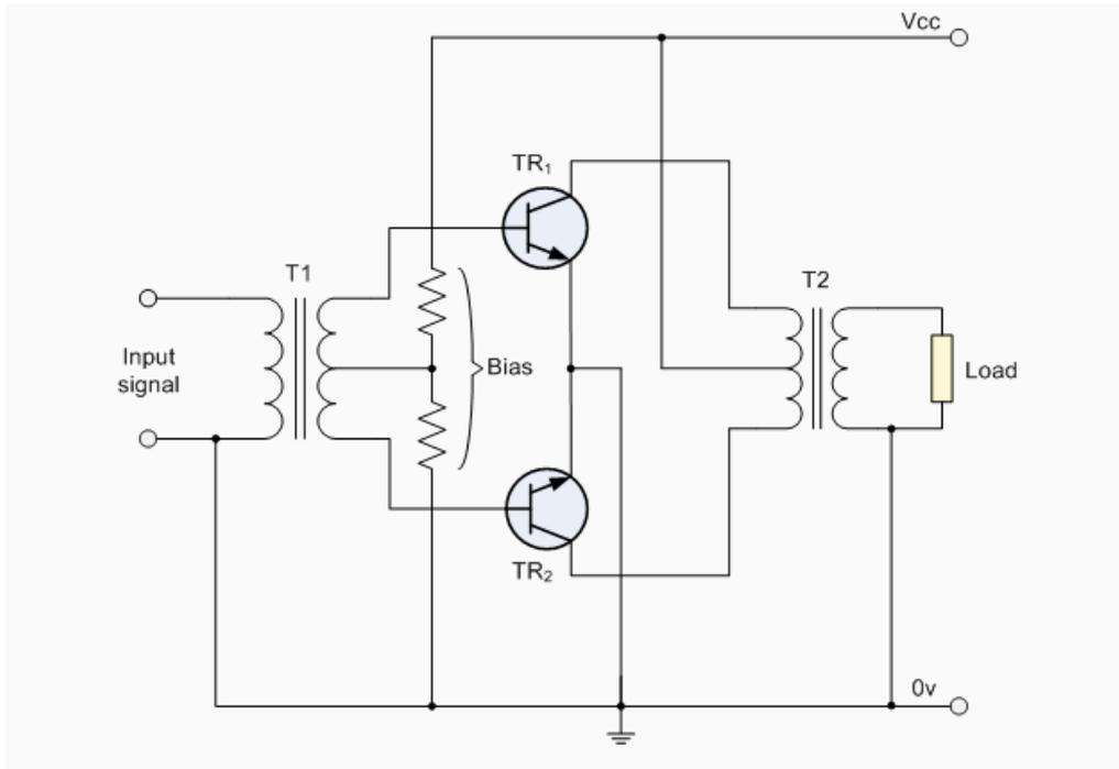
Fig3.19 Push-pull Amplifier with Pre-biasing
