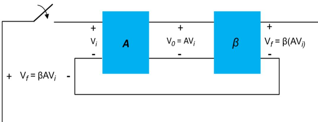
Fig 3.3 Feedback circuit used as an oscillator
