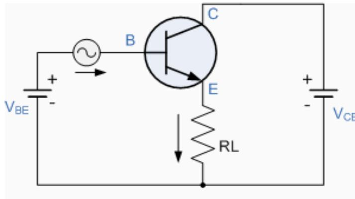
Fig 3.4 The Common Collector Amplifier Circuit
