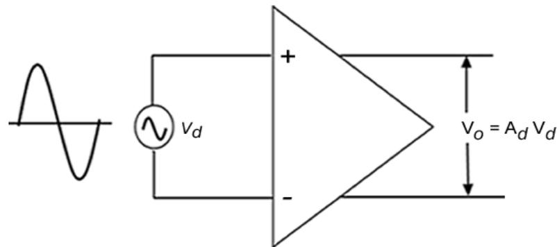
Figure 3.7 Differential-input, differential output operation.
