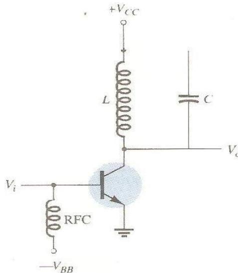
Fig 3.22 Class C amplifier circuit.
