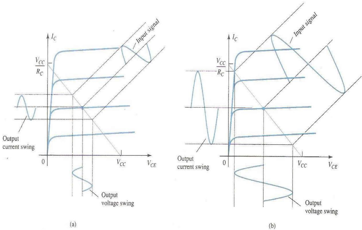
Figure 3.9 Amplifier input and output signal variation.
