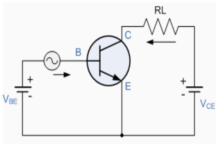
Fig 3.3 the Common Emitter Amplifier Circuit
