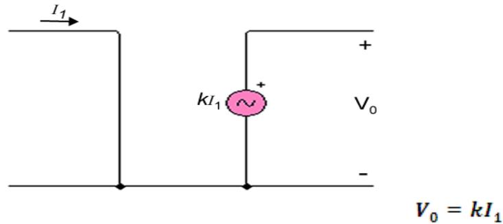
Fig 3.13 Ideal current-controlled voltage source
