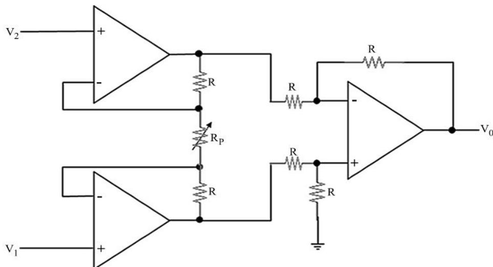
Fig 3.21 Instrumentation amplifier.
