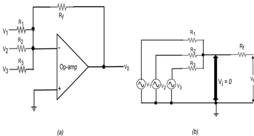
Figure 3.13 (a) Summing amplifier; (b) virtual-ground equivalent circuit.
