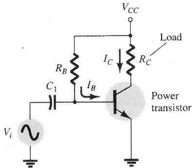
Figure 3.7 Series-fed class A large signal amplifier
