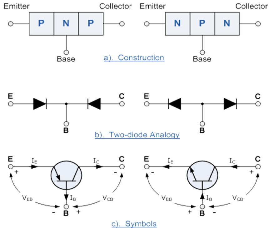
Figure 3.1: The construction and circuit symbols for both the NPN and PNP bipolar transistor are shown above with the arrow in the circuit symbol always showing the direction of conventional current flow between the base terminal and its emitter terminal, with the direction of the arrow pointing from the positive P-type region to the negative N-type region, exactly the same as for the standard diode symbol
