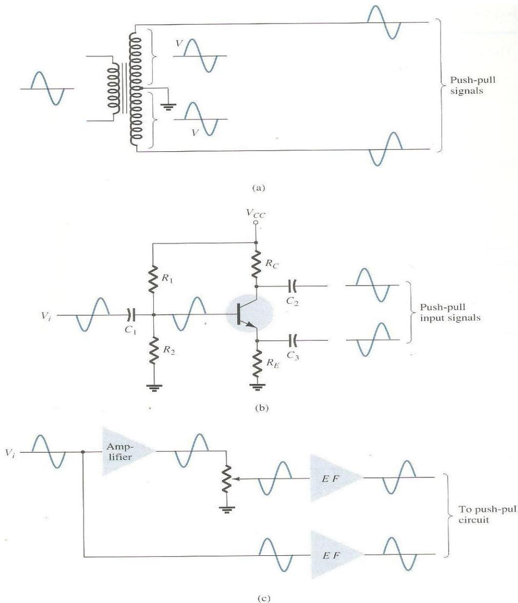
Fig 3.14 Phase-splitter circuits
