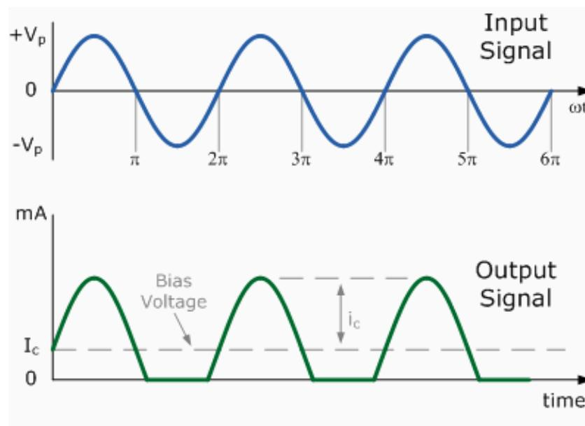
Fig3.15 Class AB Output Waveform
