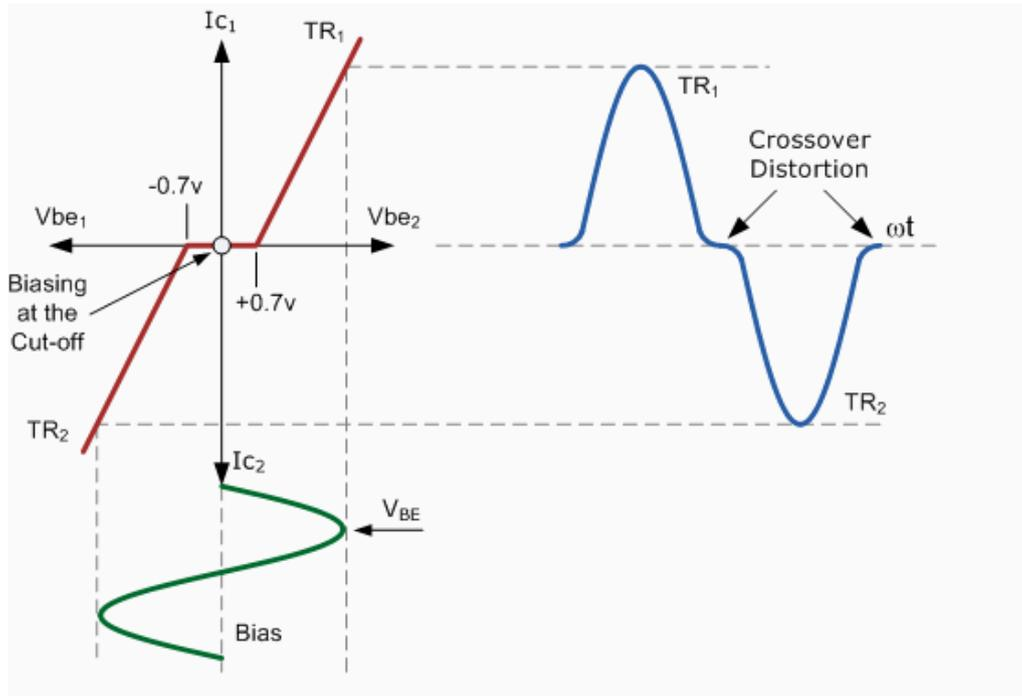
Fig 3.18 Non-Linear Transfer Characteristics
