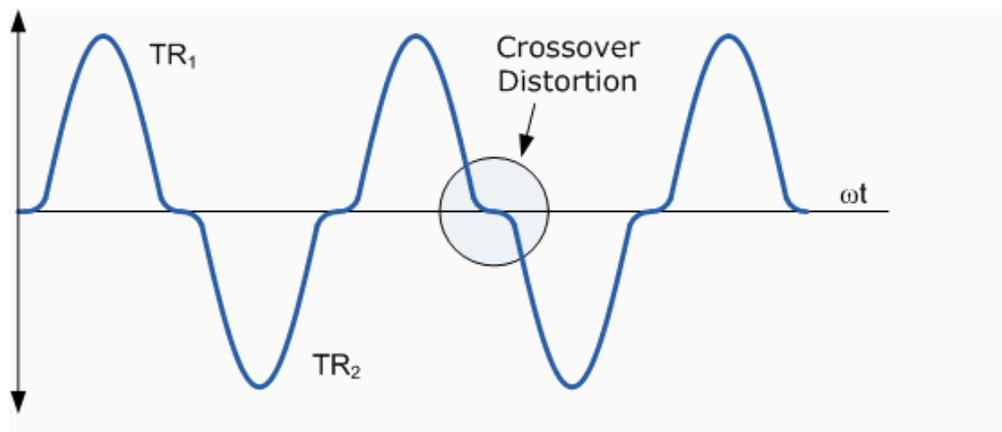
Fig3.17 Crossover Distortion Waveform
