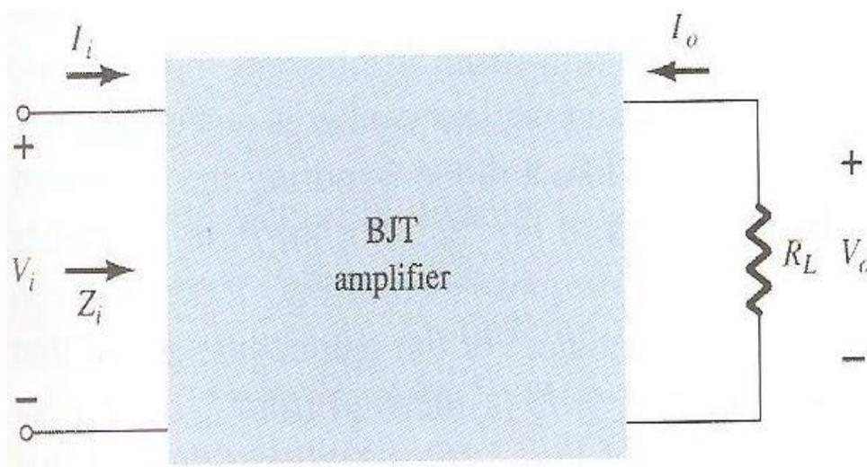
Fig 3.17 Determining the loaded current gain.
