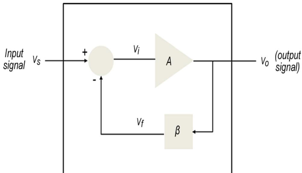
Figure 1.2- Simple block diagram of a feedback amplifier
