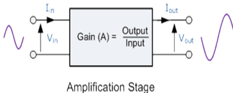
Figure 3.2: Amplifier Gain of the Input Signal
