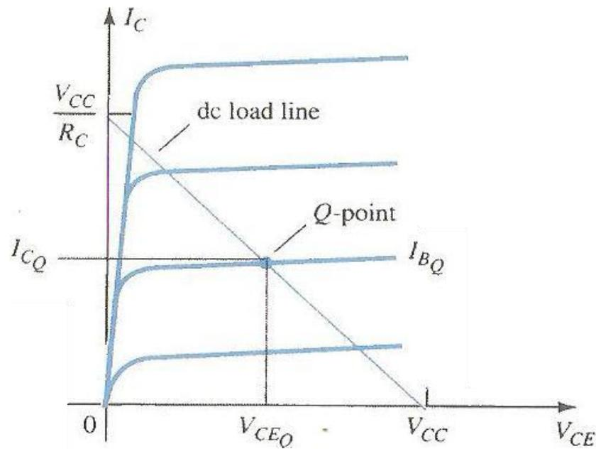
Figure 3.8 Transistor characteristics showing load line and Q-point.
