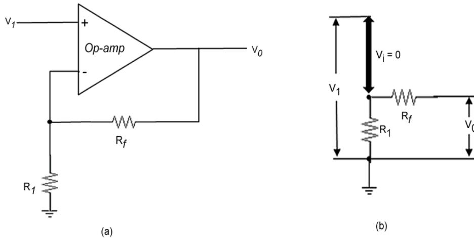
Fig 3.11 Non-inverting constant-gain multiplier
