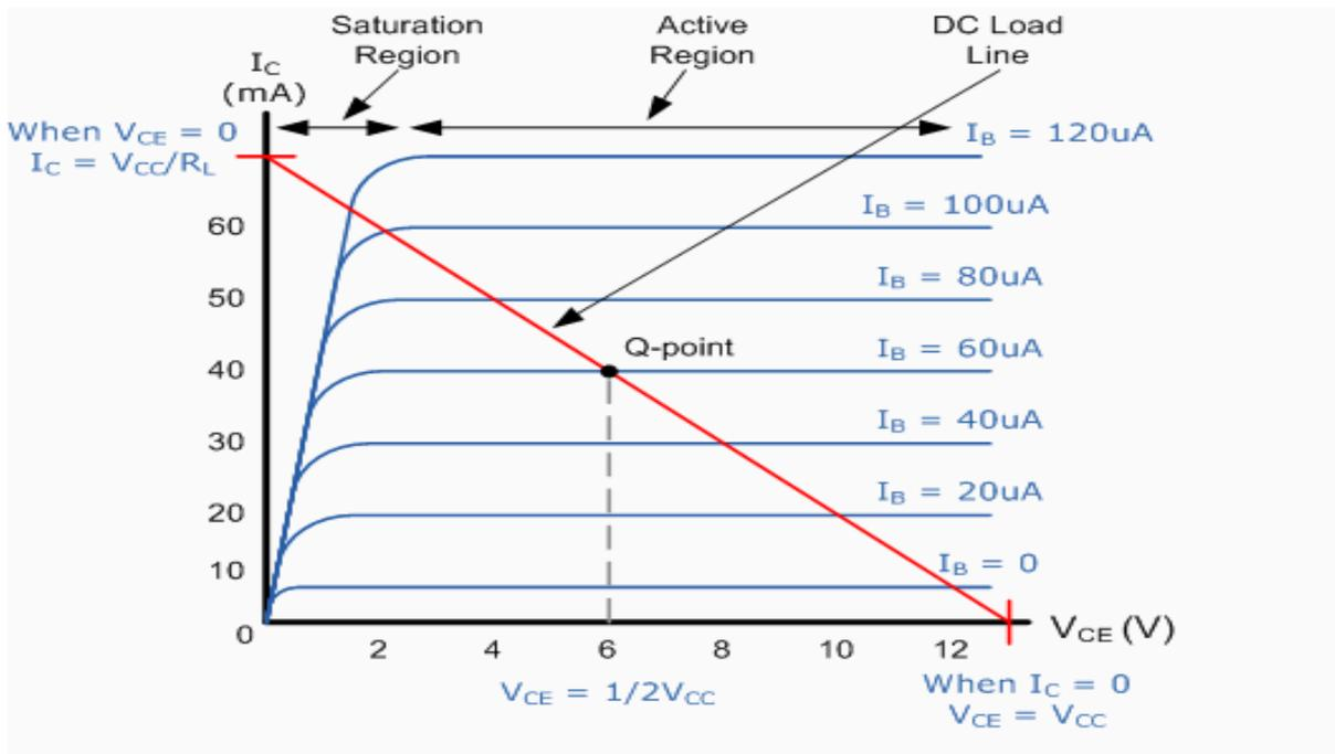
Fig 3.7 Output Characteristics Curves for a Typical Bipolar Transistor
