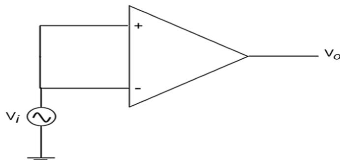
Fig3.8 Common-mode operation.
