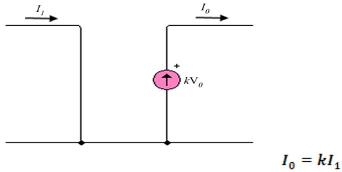
Fig 3.15 Ideal current-controlled current source
