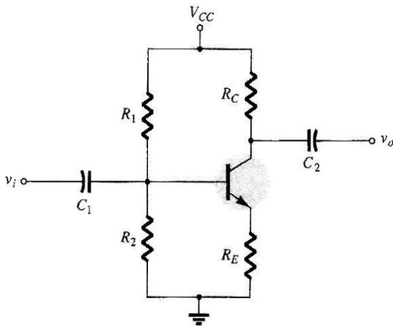
Figure 3.9 Voltage-divider bias configuration.
