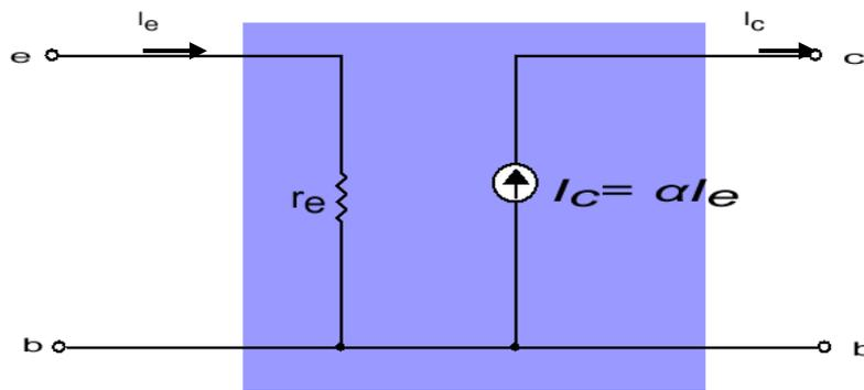
Fig 3.19 Common-base equivalent circuit
