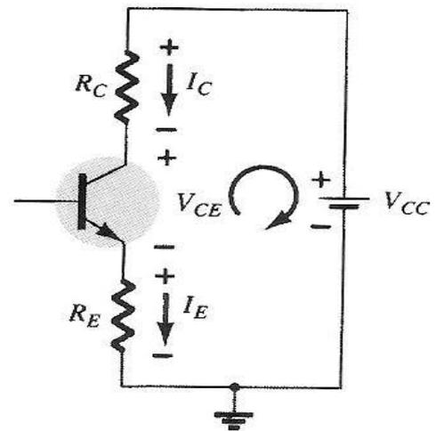
Figure 3.8 Collector-emitter loop.
