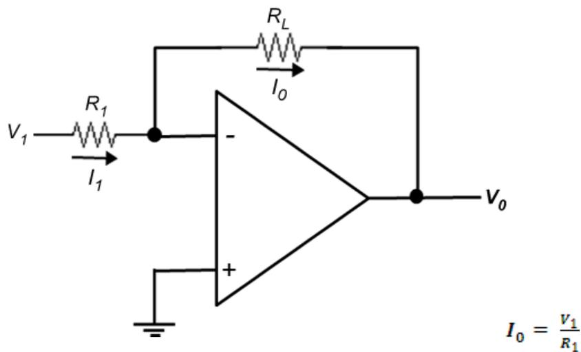
Fig 3.13 Practical voltage-controlled current source
