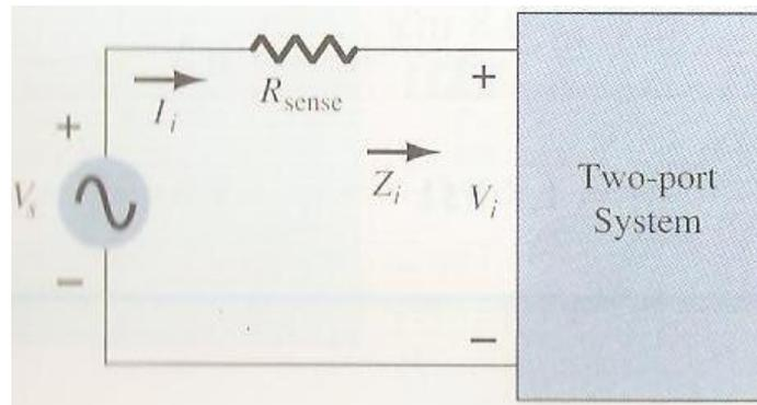
Fig 3.13 Determining  $Z_i$ .
