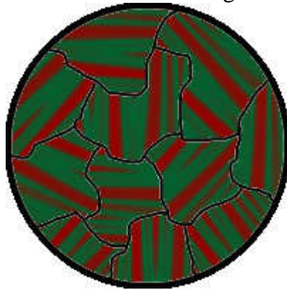
Fig. 4: Weiss domains microstructure
