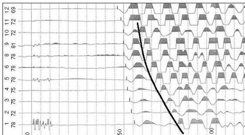
**Fig. 1.2:** Enhancement Seismograph Record showing Curved Alignment of Reflections (the thick line)
