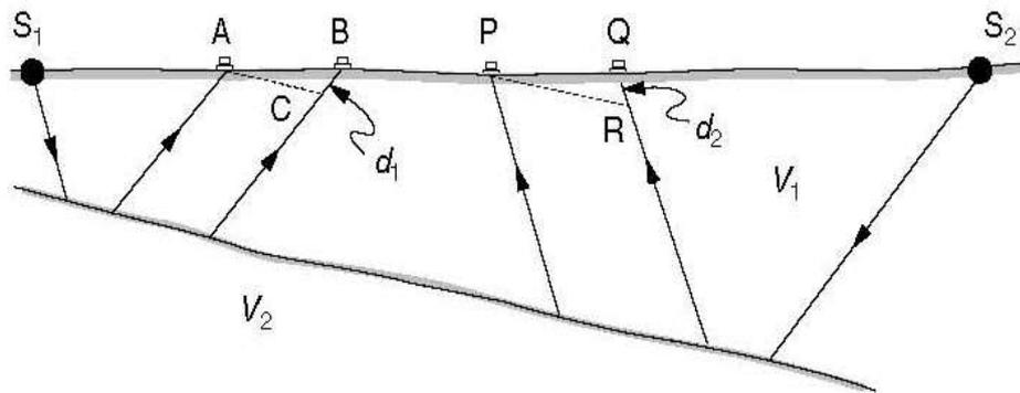
**Fig. 2.2: Refraction at a Dipping Interface**
