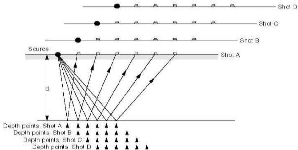
**Fig. 2.2:** CMP Schematic, for 3-fold Cover with a 6-channel System
