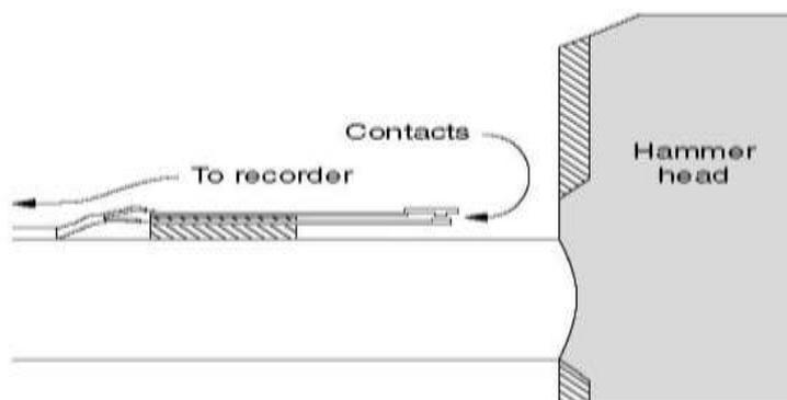
**Fig. 2.2:** “Post-Office Relay” Impact Switch on the back of a Sledgehammer Handle
