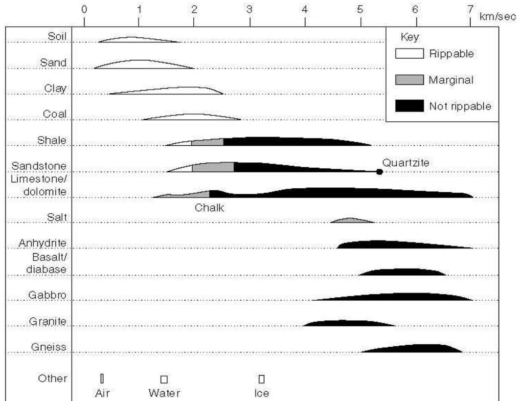
**Fig. 1.1: Ranges of P-wave Velocities and Rippabilities in Common Rocks. The Vertical axis, for each Rock type, is intended to show approximately the Relative Numbers of Samples that would show a given Velocity**
