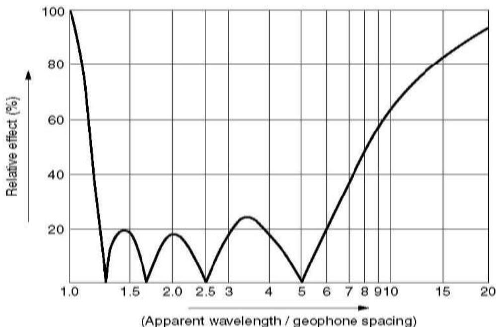
**Fig. 2.1: Relative Effect (RE) of an Array of five equi-spaced in-line Geophones**
