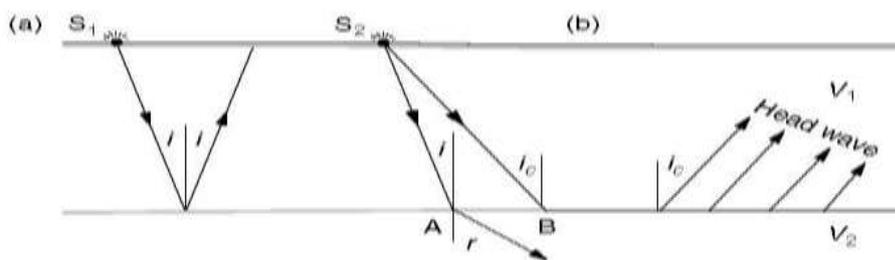
**Fig. 1.2:** (a) Reflection and (b) Refraction: Simple Refraction Occurs at A while Critical Refraction Occurs at B
