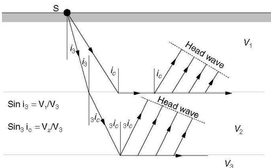
**Fig. 1.1: Critical Refraction at Two Interfaces:  $\sin i_c = V_1/V_2$**
