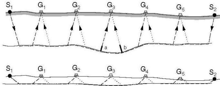
**Fig. 2.3: Effect on Travel Times of a Bedrock Depression**
