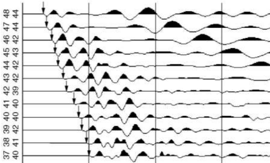
**Fig. 1.2:** Portion of a Multi-channel Refraction Record, with first-break “picks” Identified by arrows
