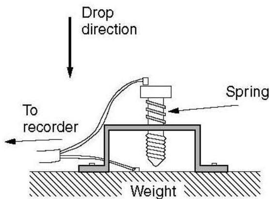
**Fig. 2.3: Weight-drop Contact Switch**
