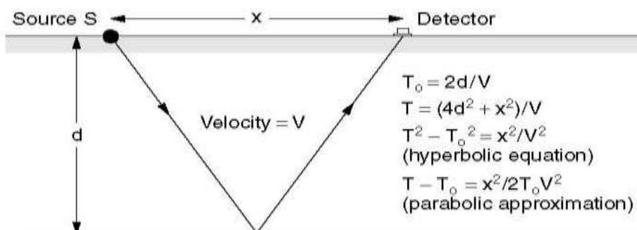
**Fig. 1.1:** Derivation of the Normal move-out Equation for a Horizontal Reflector ( $T_0$  is the normal incidence time)
