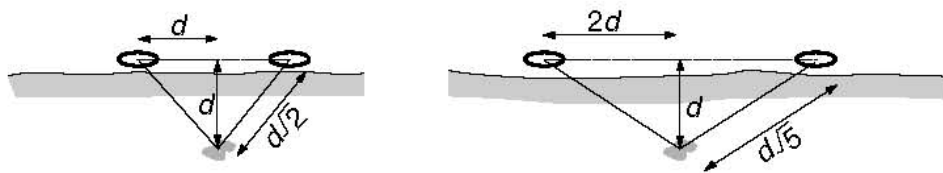
Figure 3.3 Spacing and penetration. When the two coils are moved apart, the fractional change in distance between them is greater than between either and the conductor at depth. The increased separation thus increases the anomalous field as a percentage of the primary. In the example, doubling the separation increases the coil to target distances by about 60%.
