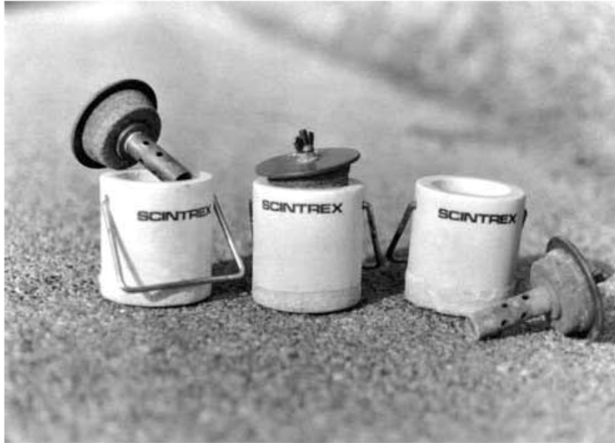
Figure 1.4 Porous-pot non-polarizing electrodes designed to be pushed into a shallow scraping made by a boot heel. Other types can be pushed into a hole made by a crowbar or geological pick.
