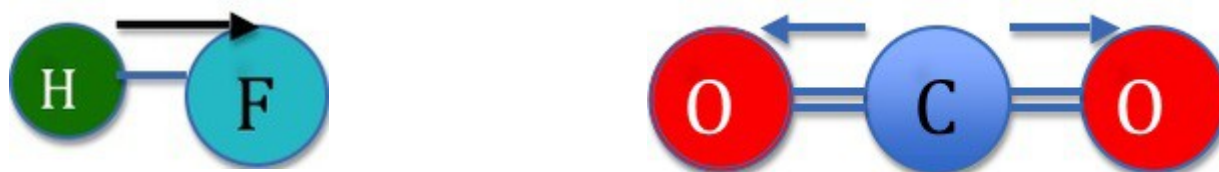
Fig. 2: Representation of dipole moment in HF and CO 2
