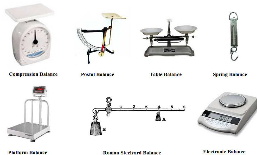
**Fig. 11: Different balances for measuring the mass of substances/objects**
