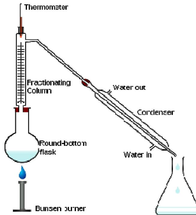
**Figure 1: Apparatus set up for Fractional Distillation**
