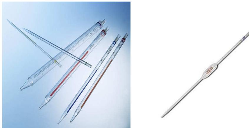
**Figure 13: Pipettes of different sizes**
