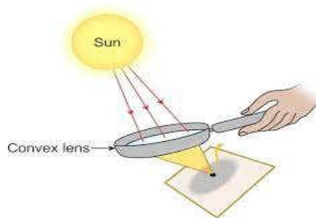
*Fig. 7:* The picture above shows how the light energy from the sun passes through the lens to a particular point on the piece of dry paper. This concentrated light energy becomes hot enough to burn the paper.
