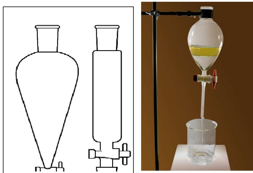
**Figure 3: Using Separatory Funnels to separate Liquids in two layers**
