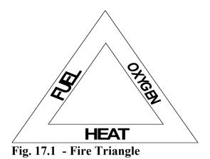
These factors are represented diagrammatically as 3 side of what is called the fire triangle. The fire triangle cannot stand if one of the factors is removed. It will collapse which indicates that fire outbreak will be impossible or could be prevented or stopped just by removing one of the factors.
