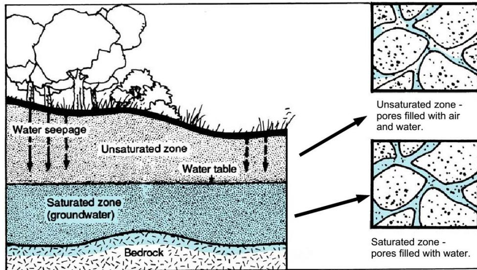
**Fig.3.1: Typical Water Table**
