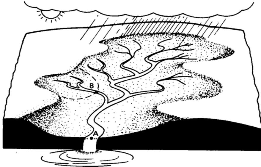
**Fig.1.1: Diagram of a Watershed**
