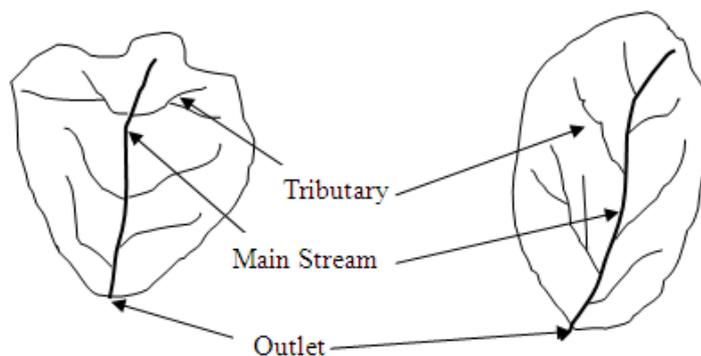
**Fig.2.1: Fan Shaped and Leaf Shaped Catchments**
