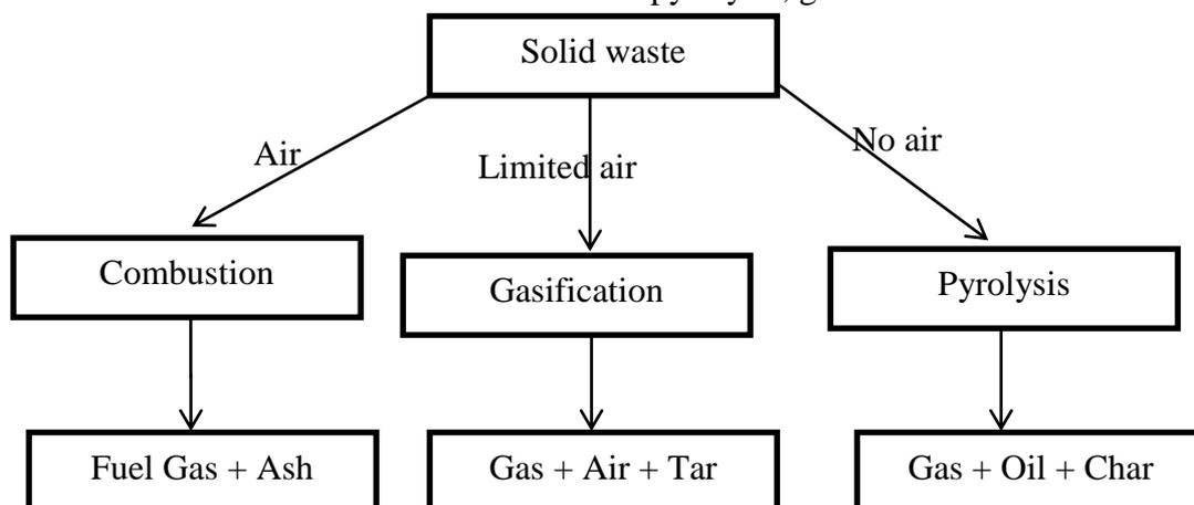
Fig 1: The main difference between pyrolysis, gasification and incineration.
