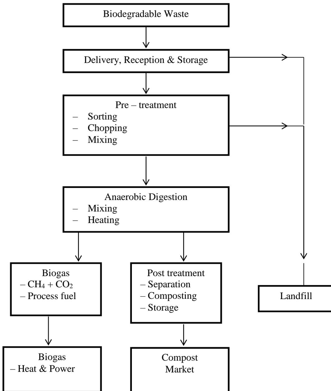
Fig 2. Schematic diagram of the anaerobic digestion process for biodegradable waste.
