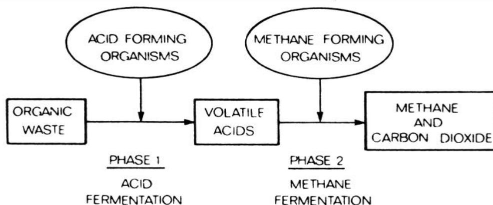
Figure 1: Methane production by microbial fermentation (Adapted from Obi et al. (2016)).
