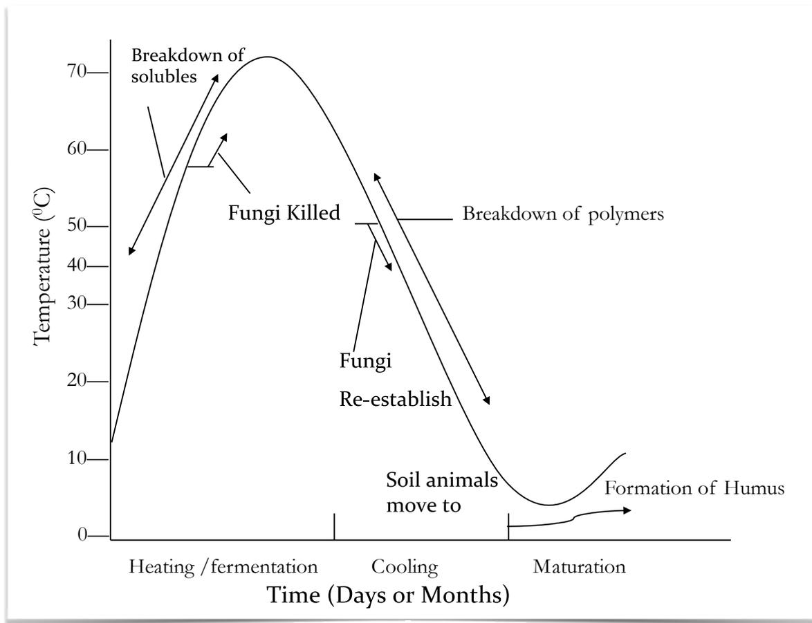
Fig 2: Temperature variation in Compost heap
