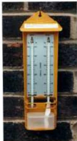
Humidity is measured most accurately with a wet- and dry- bulb thermometer
