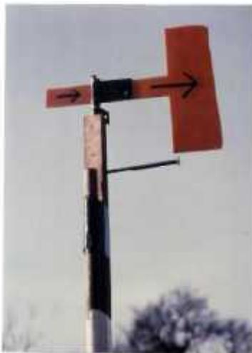
A simple home-made weather-vane can measure wind speed and indicate wind direction
