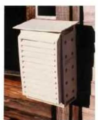
Ordinary spirit-in-glass thermometer. This simple louvered thermometer screen is available as a kit
