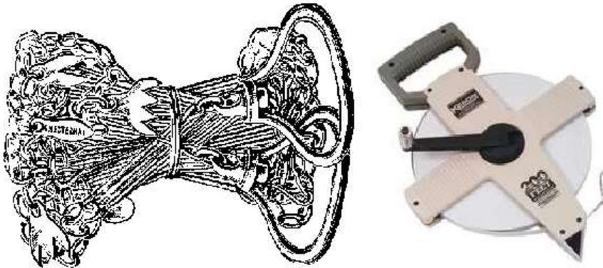
Figure 11: Gunter's chain and measuring tape.
