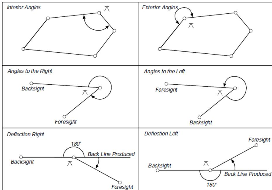
Figure 12: Types of Angle Measurements.
