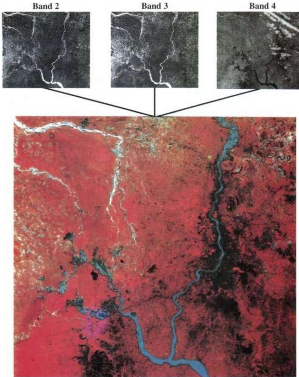
Figure 25: I RS- 1 0 LISS-11i FCC image (bands 2, 3, 4) and corresponding Black and White Images of band 2, band 3 and band 4 data of path .108, row 56, showing Calcutta and Surrounding Areas.
