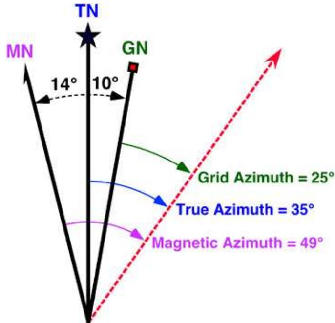
Figure 4. Declination difference between Grid, True, and Magnetic North.
