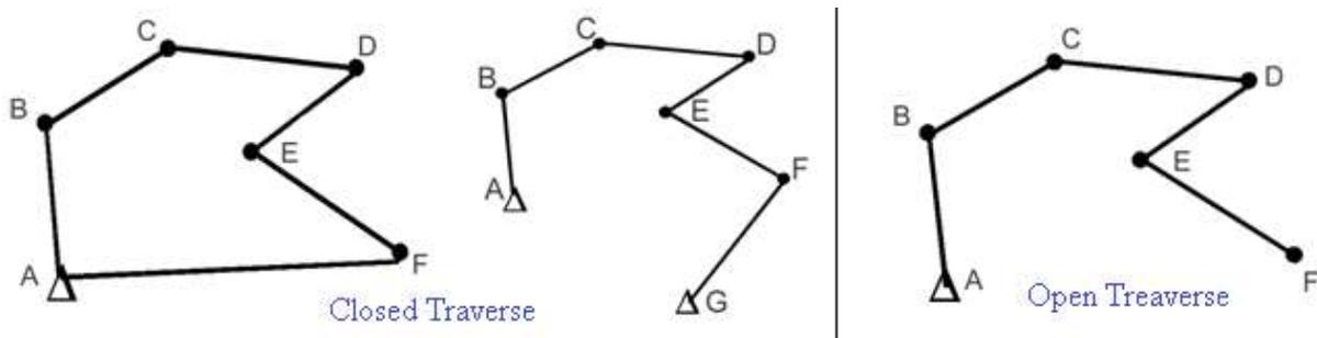
Figure 13: Examples of survey traverses.
