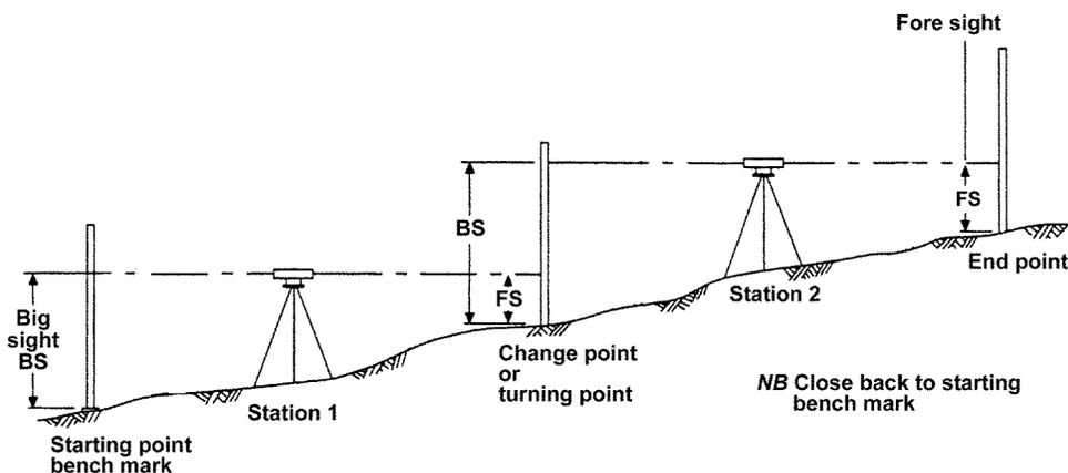
Figure 16. Method of traverse levelling.
