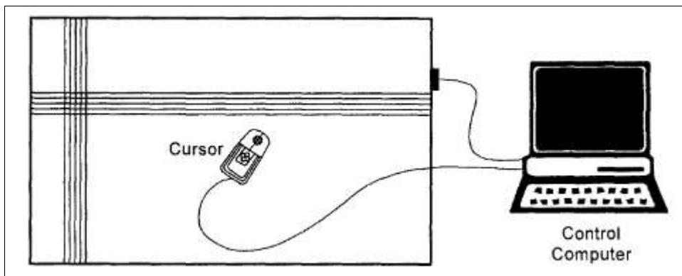
Figure 27 Contemporary wires embedded tablets digitizer.
