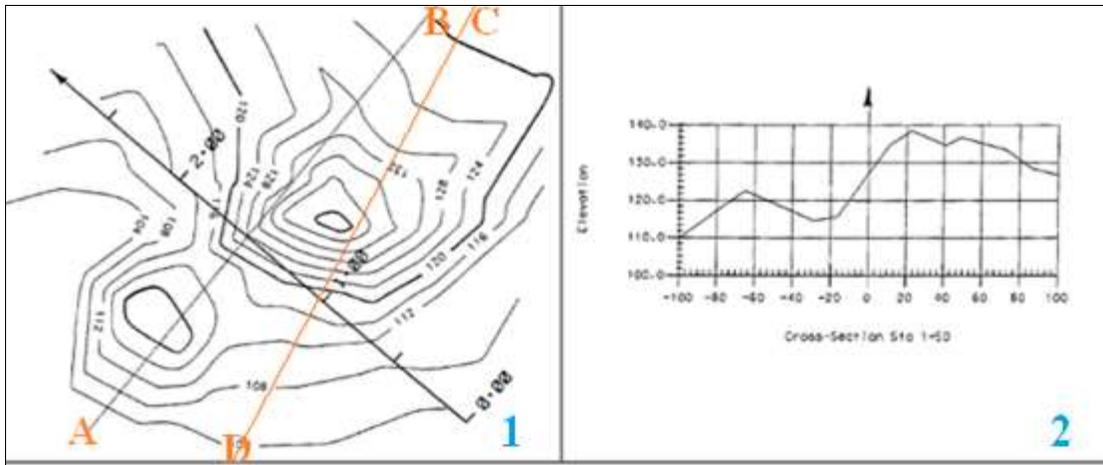
Figure 32 Terrain cross section cutting.
