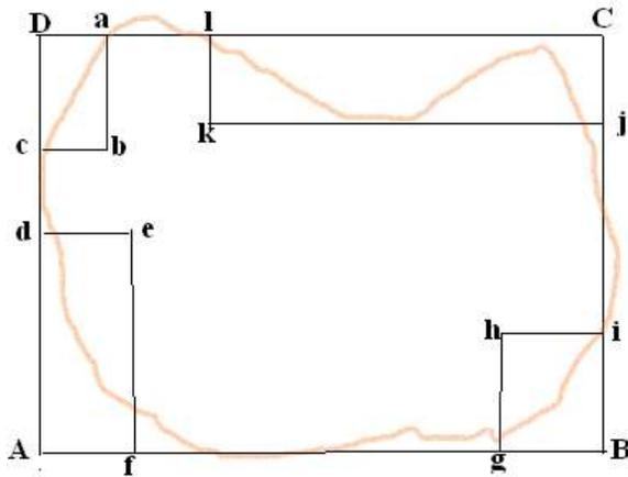
Figure 5. The use of rectangles to calculate irregular area on maps.
