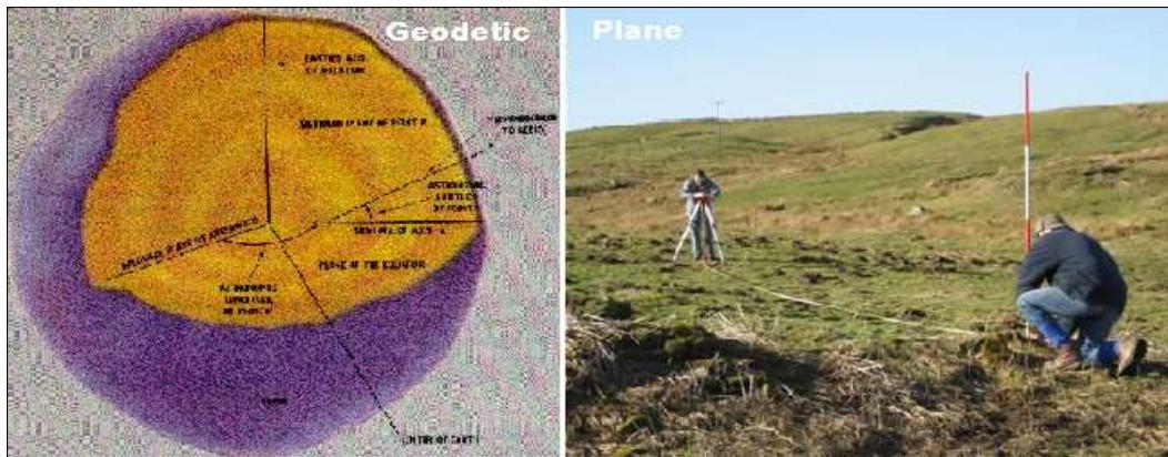
Figure 10: Geodetic and Plane surveying.
