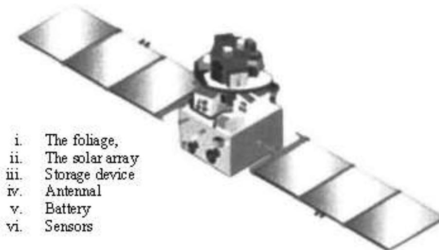
Figure 19. Outer space satellite components
