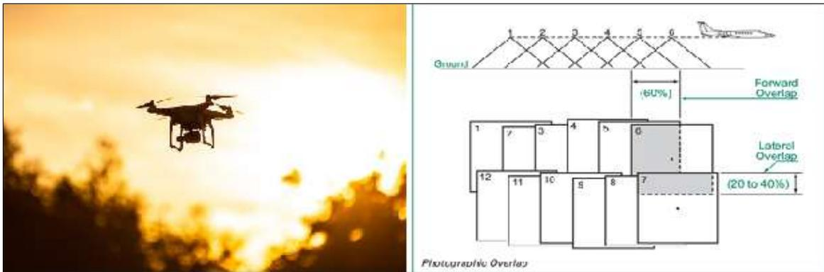
Figure 17: Photo flight line and overlaps
