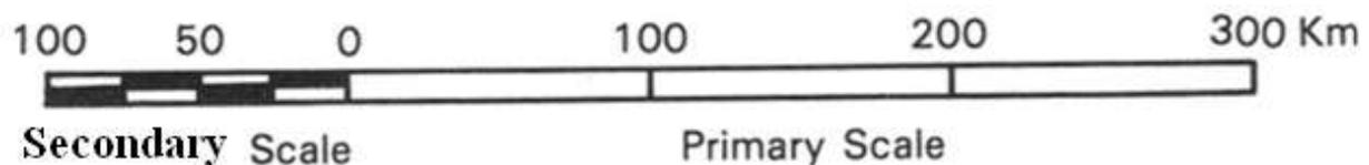
A linear scale is often made up of two component parts namely the primary subdivisions and the secondary subdivisions. The 'primaries' are on the right hand side of the zero while the 'secondaries' are on the left hand side. While the primaries are subdivided into kilometres (or miles), the secondary are subdivided into smaller units such as metres (or furlongs).
