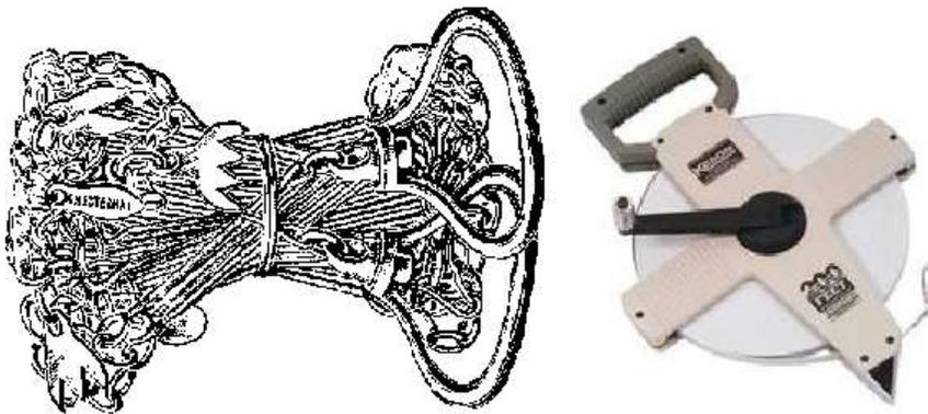
Figure 11: Gunter's chain and measuring tape.
