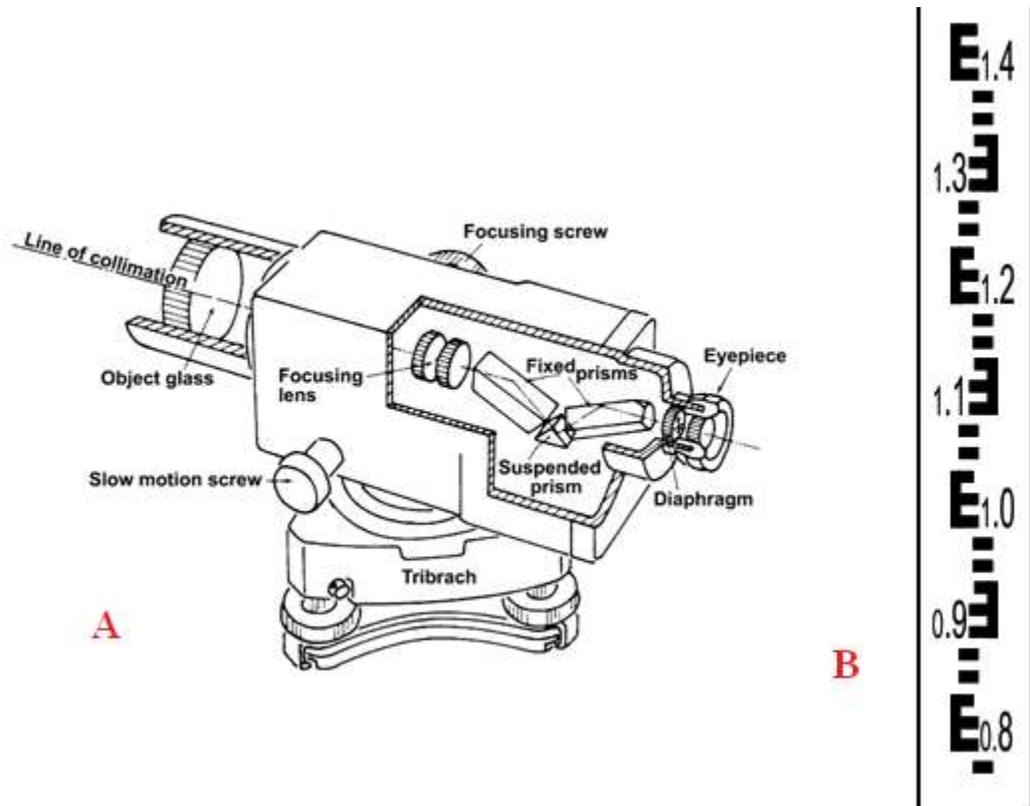
Figure 15. WILD automatic level with fixed suspended prisms and levelling staff
