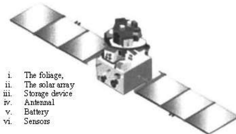
Figure 19. Outer space satellite components
