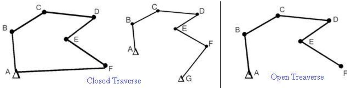
Figure 13: Examples of survey traverses.
