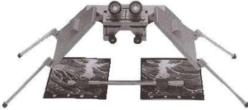
Figure 18; Mirror Stereoscopic viewer
