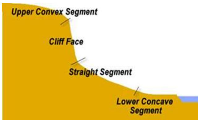
Figure 8 Show the element of slope
