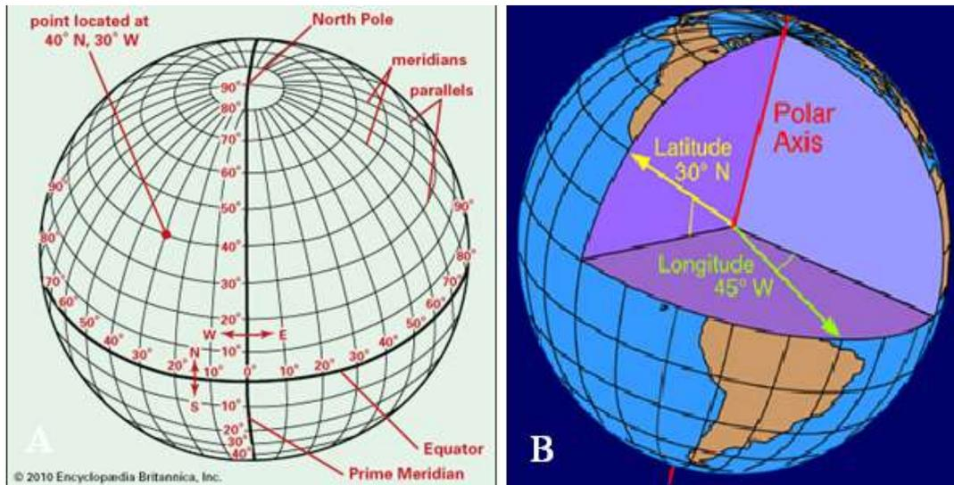
Figure 1a, b: Measurement of latitude and longitude relative to the equator, the Prime Meridian and the Earth's rotational or polar axis.
