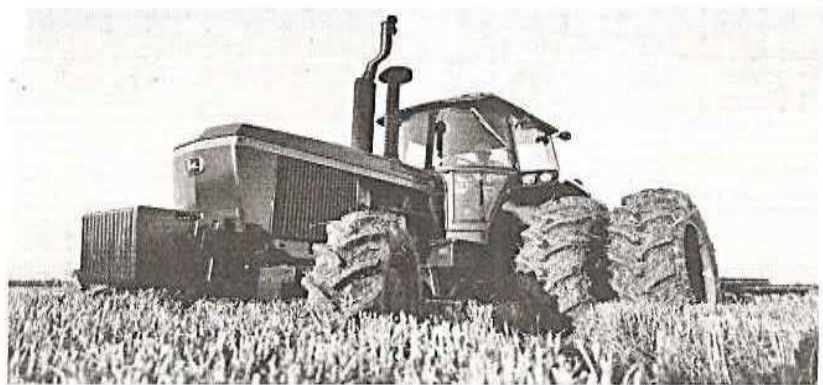
FIG. 16-7. Two-wheel drive tractor with optional front wheel power drive. (Courtesy Deere and Company)
