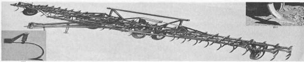
Fig. 18-27. Pull-type field cultivators have become very popular secondary tillage tools for field finishing or seedbed preparation working 2 to 5 in [50 to 125 mm] deep. Outside wings fold for transport and flex for even penetration across the full width of the unit. (a) Sharks are spring-cushioned (insert) for vibrating action and trash removal. Shank points are 1\frac{3}{4} \times \frac{1}{4} \times 11 in [44.45 \times 6.35 \times 279.4 mm] and are used for shattering crust ahead of planting. (b) V-sweeps are 4 to 12 in [101.6 to 304.8 mm] wide and are used for weed control, leaving crop residue on or near the surface. (Deere & Co.)
