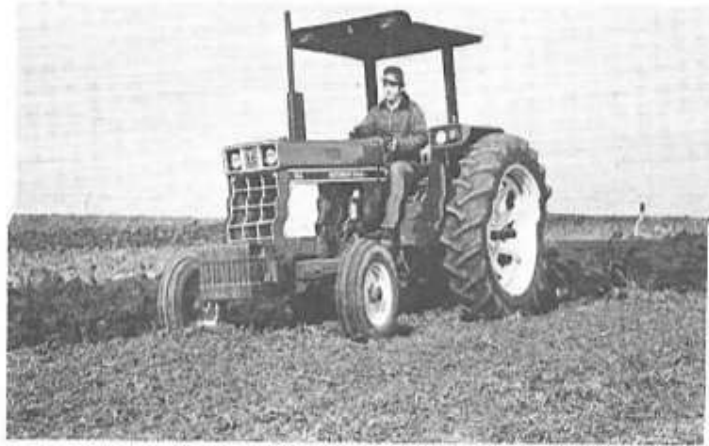
FIG. 16-3. Utility tractor, 65 h.p.; can be used for row crops. (Courtesy International Harvester)
